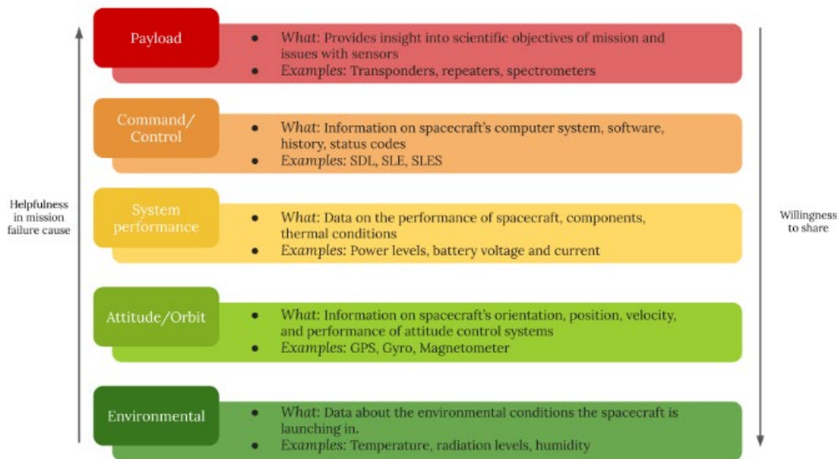
Figure 1: Satellite data categories ranked based on helpfulness in mission failure detection and willingness to share
