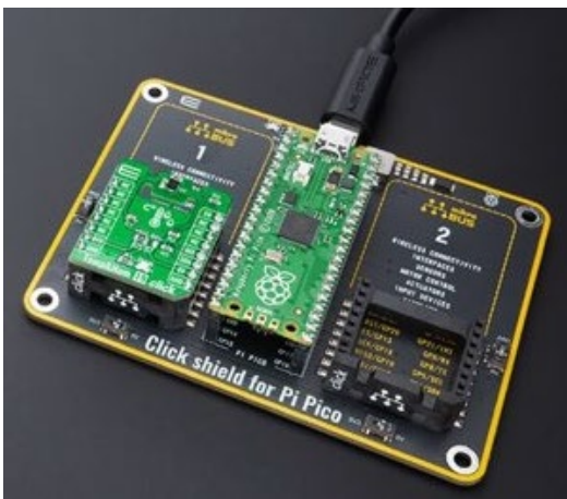
Figure 8: PI Pico Microcontroller Click Shield (4)
