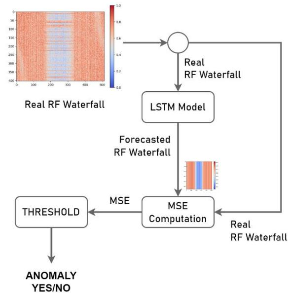
**Figure 9: Anomaly detection system architecture, with LSTM models.**
