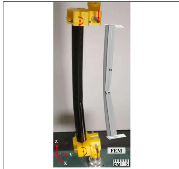
Figure 13: Eccentric Buckling of UTHS Boom
