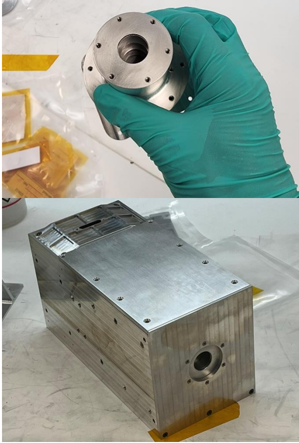
Figure 1 (Top) HERT sensor head; (bottom) HERT whole assembly.
