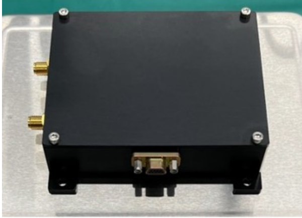
Figure 7: Engineering model of the store and forward radio.
