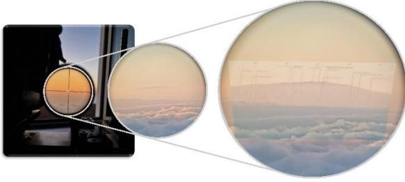
**Figure 7: Alignment procedure of the LCT toward its target in La Palma. The first picture shows the view from the finderscope. The second shows the view from the finderscope of the island of La Palma. The last picture superimposes a landmark panorama<sup>20</sup> over the island to show the exact position of JKT.**
