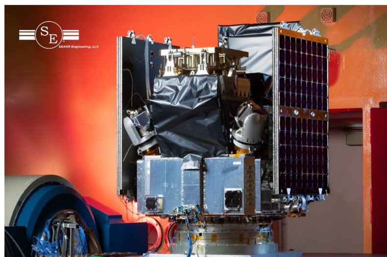
Figure 3: Fully Integrated Blackjack Space Segment Ready for System-Level Testing
