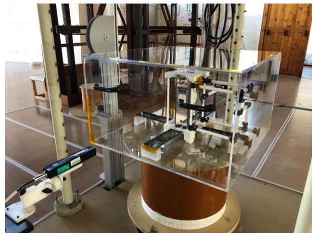
Figure 4: Test setup for residual magnetic moment measurement
