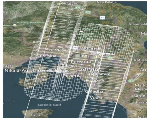
**Figure 13. Swath-Extension simulation. The satellite performs various parallel tracks over the target when passing over it.**
