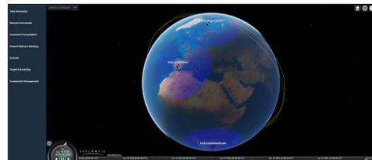
**Figure 16. MCS main screen. The satellite position activated targets and ground stations active are represented. Satellite can be propagated back and forward manually.**
