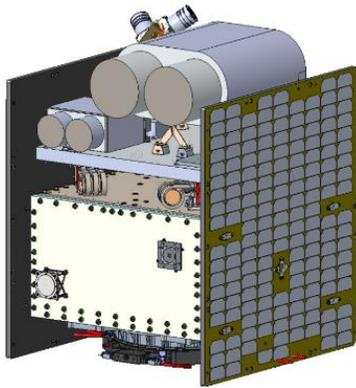
**Figure 28. GARAI satellite render in stowed position.**
