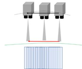
**Figure 10. Scanning acquisition mode representation. The imager is pointing at a fixed off-Nadir angle while acquiring at high FPS.**
