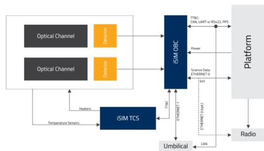
**Figure 24. Functional block diagram showing external interfaces with satellite platform.**
