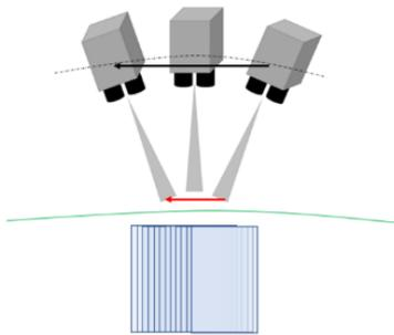
**Figure 11. Backscanning acquisition mode representation. The imager adjusts its pointing to reduce the sensor ground velocity while acquiring at higher exposure time.**
