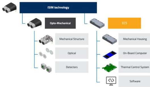
**Figure 22. iSIM imager subsystem breakdown.**
