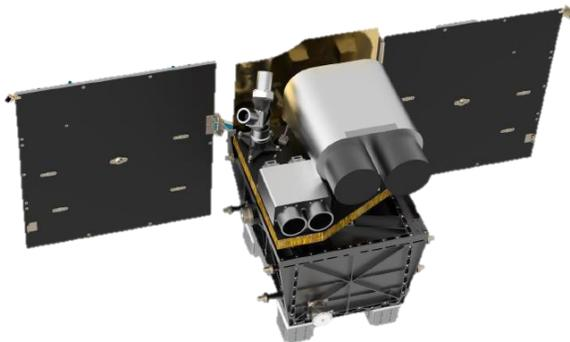
**Figure 1. GARAI spacecraft render. Featuring OHB Sweden Microsatellite platform and SATLANTIS payload.**
