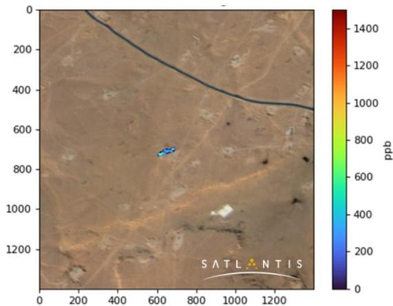
**Figure 5. Example of detection and quantification of methane emissions in Algeria desert. Performed by an iSIM-90 imager onboard a 16U-CubeSat platform.**
