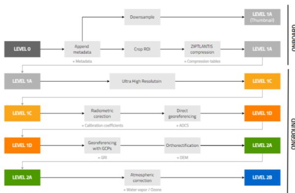
**Figure 17. Data Processing pipeline schematic.**
