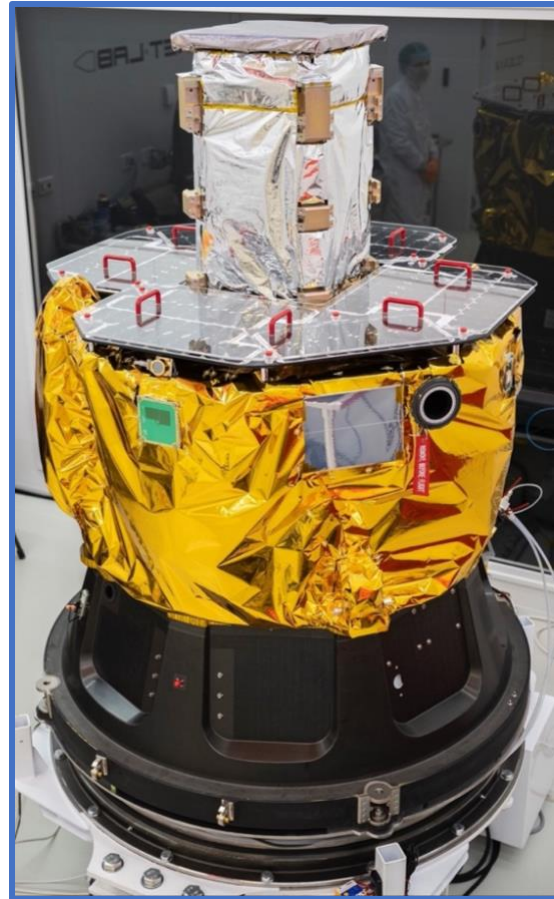
Figure 2: The CAPSTONE Spacecraft/Dispenser - Lunar Photon (gold MLI) Integrated Stack
