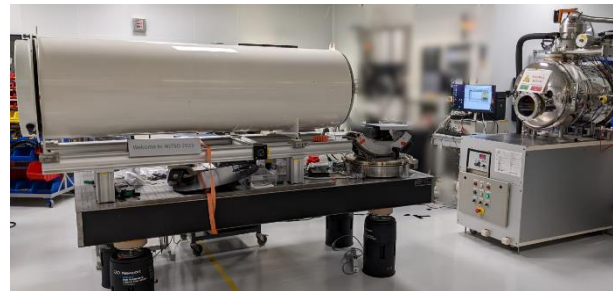
Figure 20. MTF collimator in front of the TVAC
