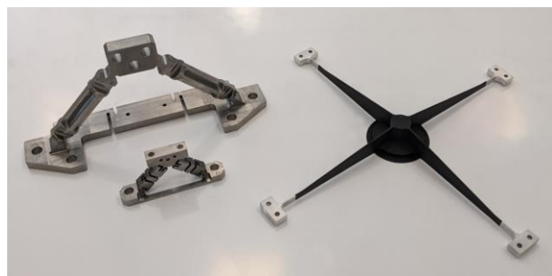
Figure 9. Bipods flexures and external baffle extra obscuration
