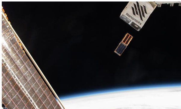
Figure 18: BurstCube (the Cubesat down and to the left) being deployed from the ISS with SNOOPI. (Credit: NASA/Matthew Dominick)
