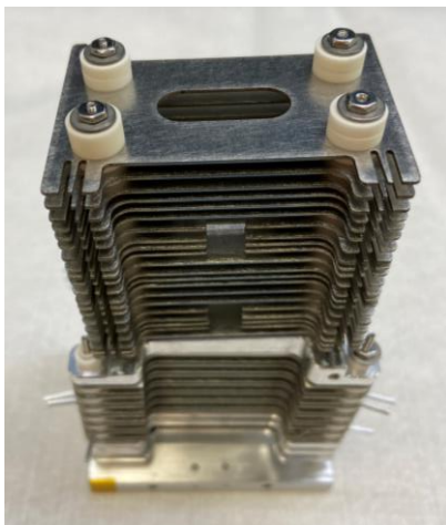
Figure 5. Photo of the orthogonal accelerator optics with 4 degree bend. Source provides extraction, acceleration, focusing and deflection.
