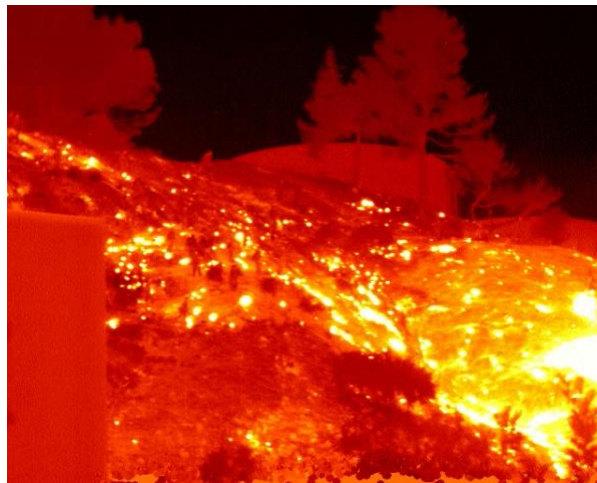
Figure 2. This image shows a wildland fire as seen from a standard 1-5.5 micron mid-wavelength infrared (MWIR) camera. Most of the pixels which detect the flaming fire are saturated due to the overwhelming MWIR signal from the fire. The overwhelming signal quickly saturates the well depth of the read out integrated circuit of the focal plane array.
