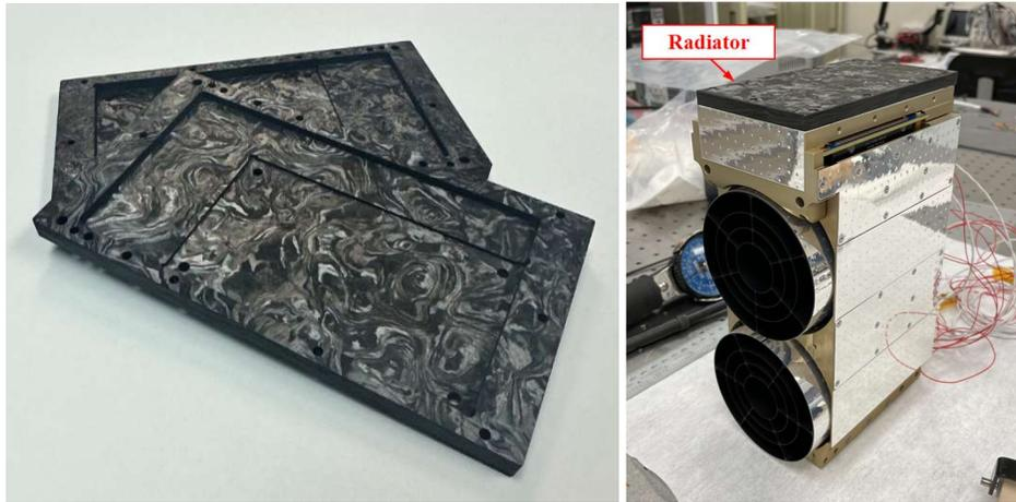
**Figure 6: Left - Carbon Fiber Radiator, Right – Radiator Installed On Deep Purple Payload**
