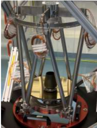
Fig. 14. Metering Structure, Optical Tube Assembly
