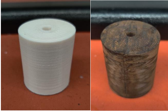
Figure 10: ABS Fuel Grain Before (left) and After (right) Catalyst Infusion
