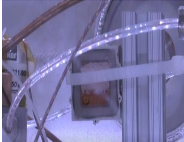
Figure 5. Vapor transfer testing using clear polymer tubing for visualization.
