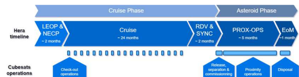
Figure 17: CubeSats operational phases and Hera timeline
