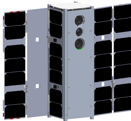
Figure 1: BeaverCube II 3U Cubesat.
