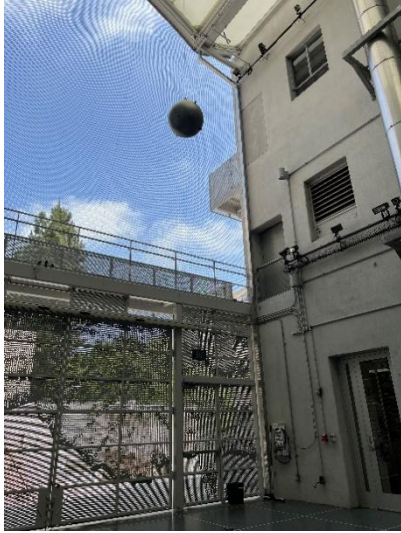
Figure 16: CAST lab 2D radar testing in range and elevation test set-up. Target at various range heights.
