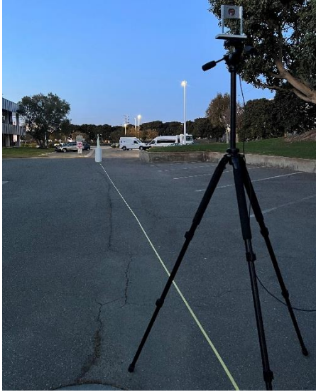
Figure 10: Parking lot 1D distance test set-up, sphere on Styrofoam stands.
