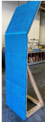
Figure 25: Portable absorber wall, with pyramidal absorber
