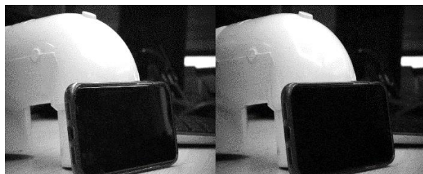
Figure 30: Using the FLIR Blackfly polarized camera to reduce glare seen on reflective surfaces. The minimum value is selected from each super-pixel, producing the glare-reduced image seen on the right.
