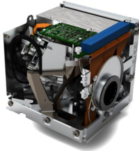
Figure 1: A Render of the CubeCAT Lasercomm Terminal, Fitting in a 1U Standard Volume
