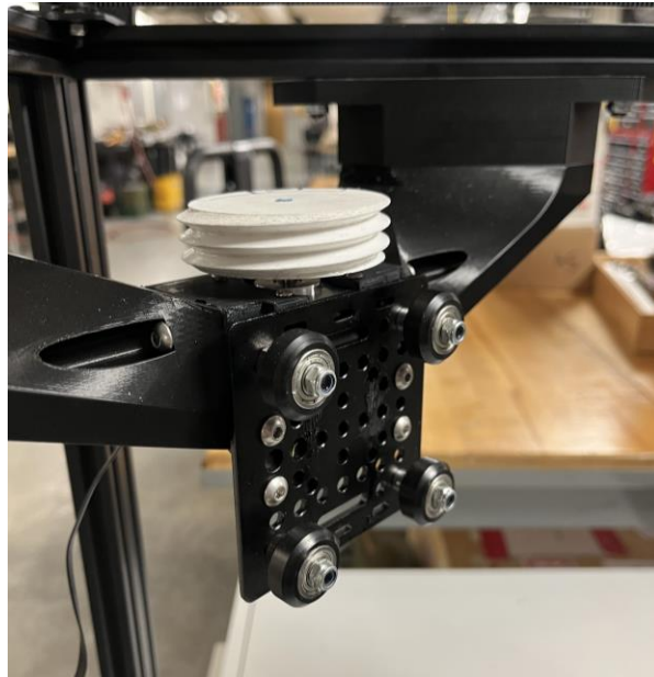
Figure 4: Z Mechanism with Guide Wheels and Worm Mounted to Printer
