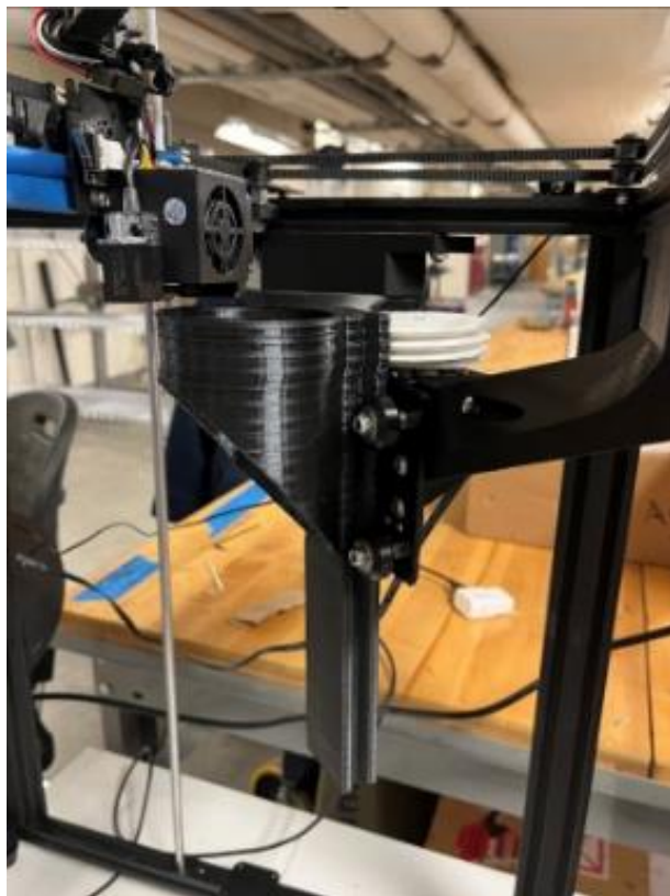
Figure 9: System Printing 125mm Extended Track with Attached Cylindrical Space Station
