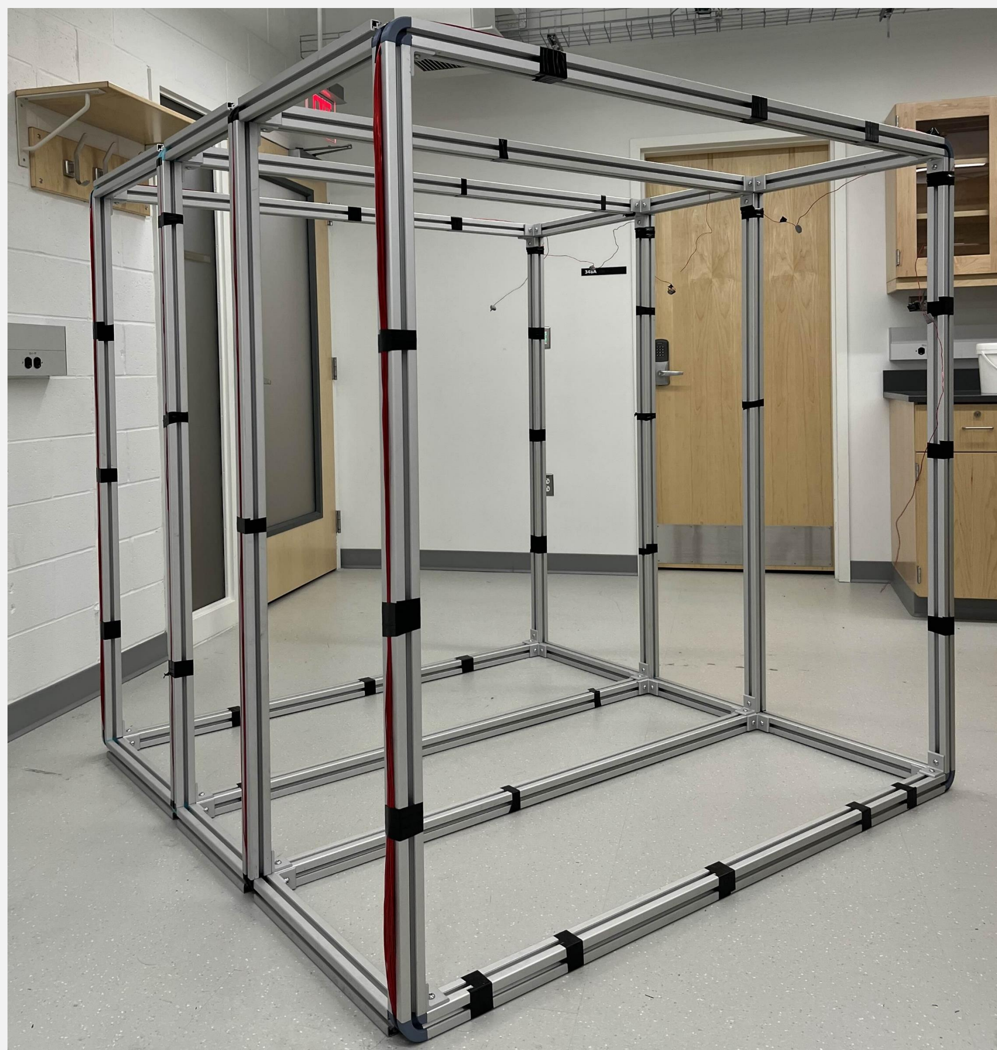
Figure 2: One axis (4 coils in series) of the Merritt Cage
