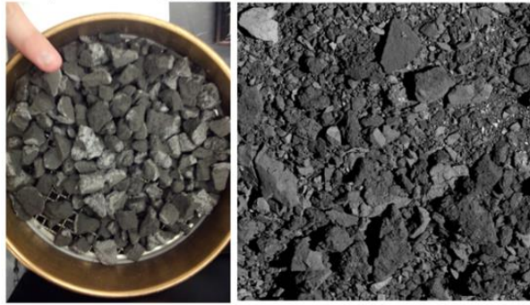
Figure 1 Sample material prepared for our investigation (cm-sized grains, left) compared to regolith at the surface of asteroid Bennu as imaged by the OSIRIS-REx mission (right). While the scale of both pictures are different, we show that our simulant samples represent well the grain shape found on asteroids.
