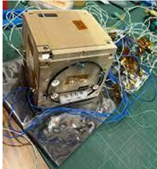
Figure 14: LignoSat Prototype measuring only 10 square centimeters [8].
