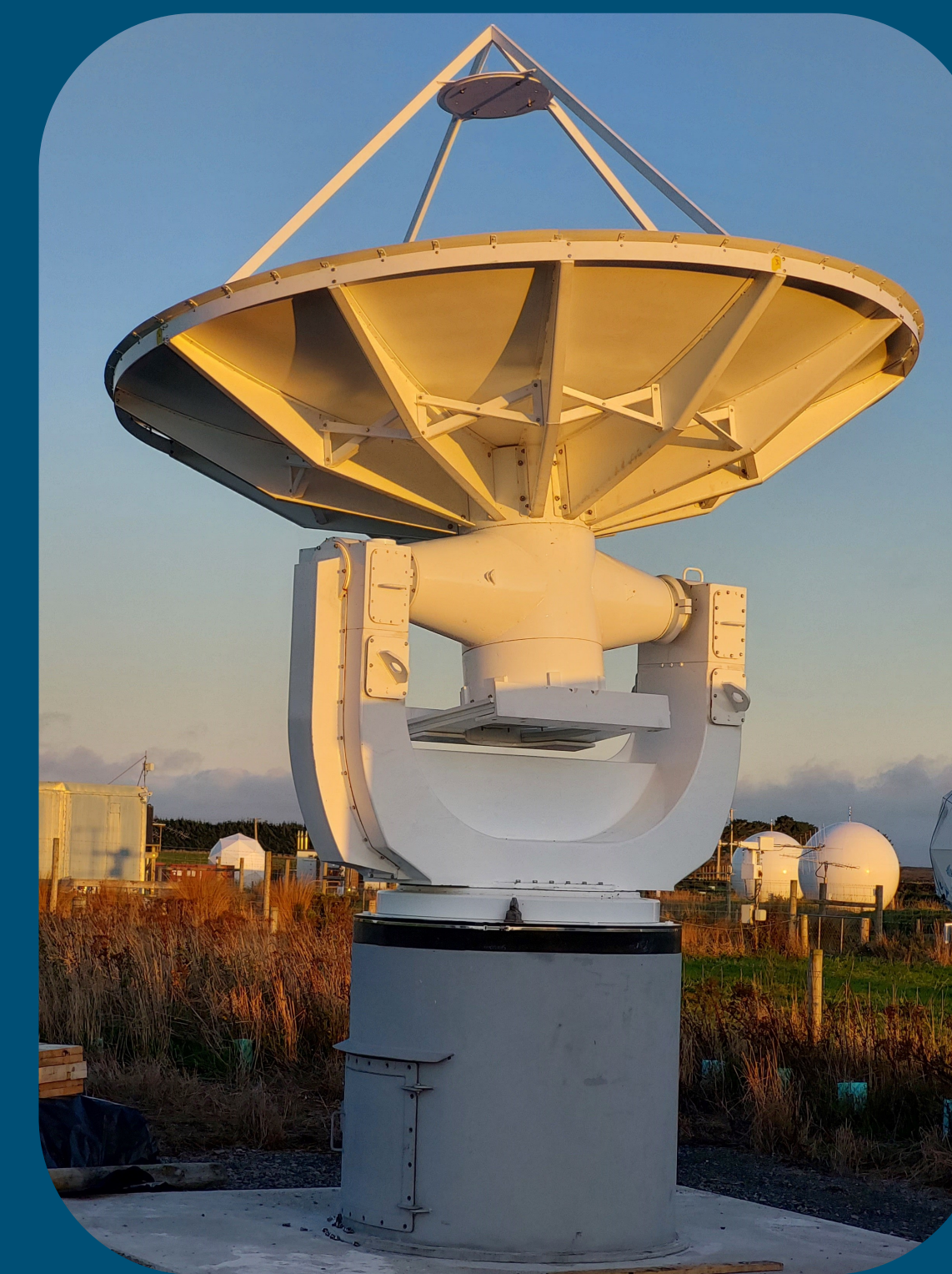
Figure 5 & 6: Measurements provided in this poster were taken on the pictured 400MHz Yagi antenna (AWA-2) and 3.7m S-/X-Band parabolic antenna (AWA-4).
