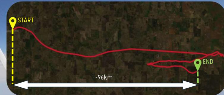
Flight path of HAB-02 over Merredin, Western Australia. Reconstructed from radiosonde data.
