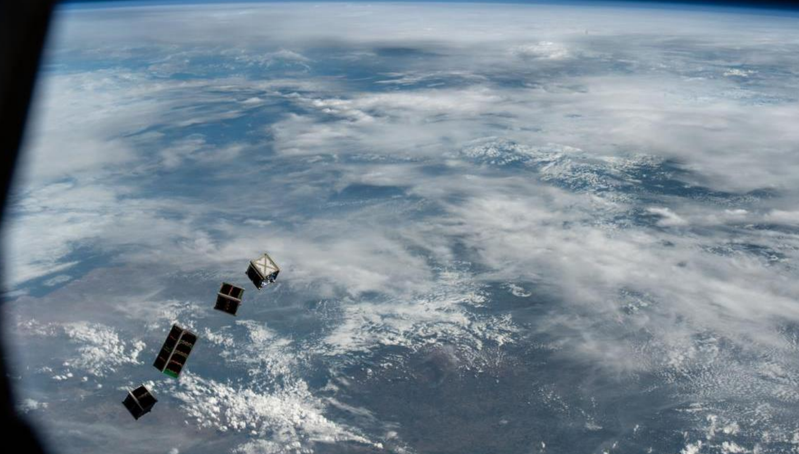
Above: a set of four CubeSats - two from Japan, and one each from Uganda and Zimbabwe - are deployed into Earth orbit for a variety of scientific studies and technology demonstrations from a small satellite deployer on the outside of the Kibo laboratory module as the International Space Station orbited 264 miles above Namibia, Dec 2022
