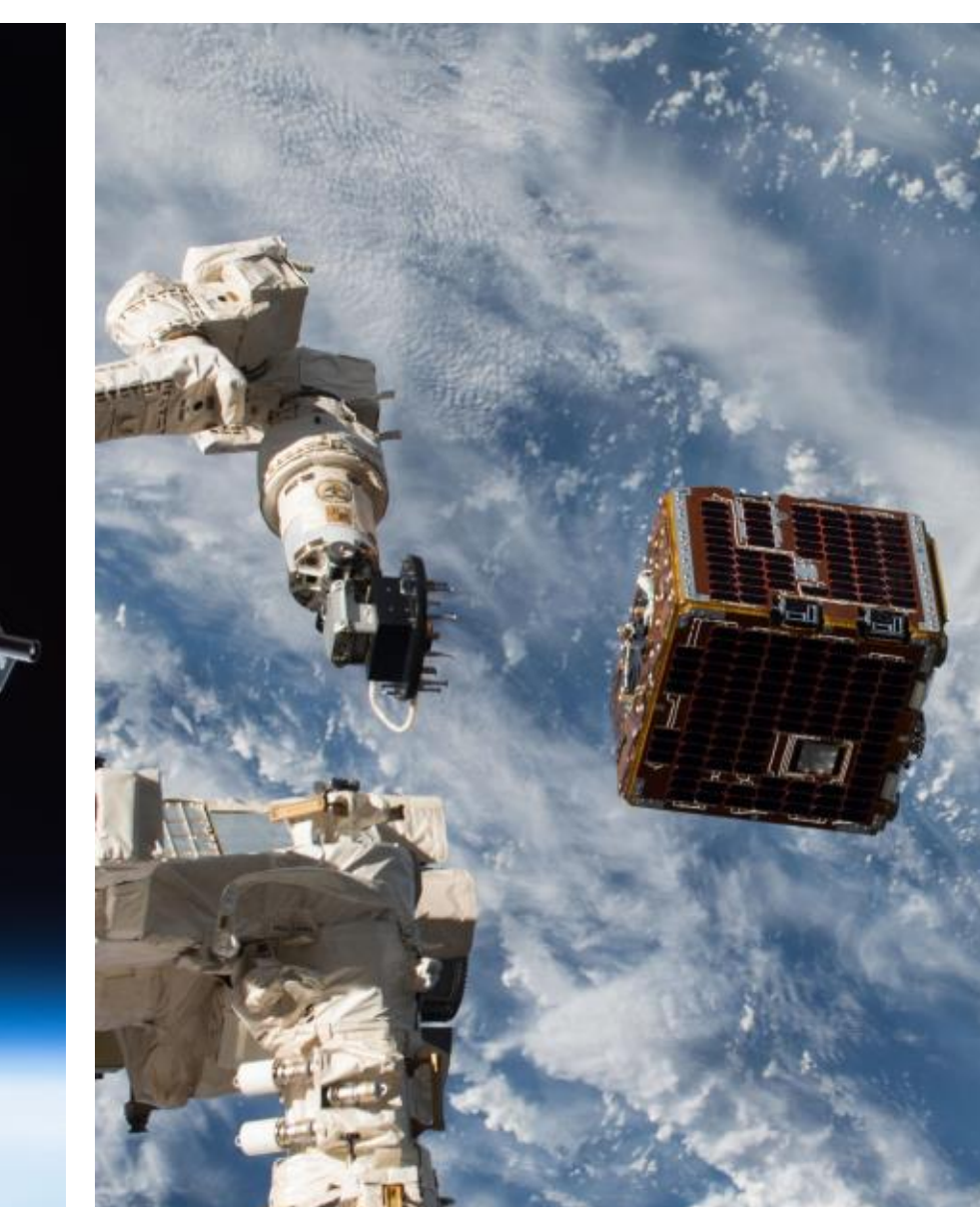
Left: Cyclops deployer with SpinSat preparing for release, Nov 2014 Right: Deployment of the NanoRacks-Remove Debris Satellite using the NanoRacks Kaber MicroSat Deployer, Jun 2018
