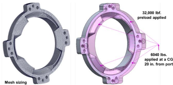
Figure 5: Simulation Setup and Mesh Sizing for the Cup-cone Interfaces
