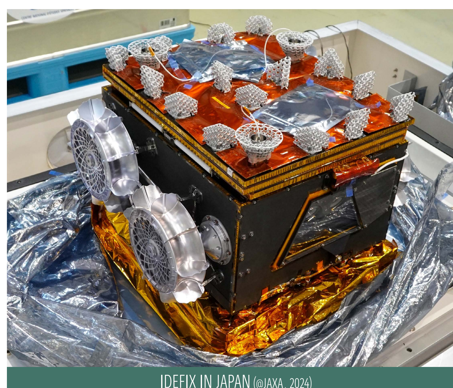
THE MAIN ROVER INTERNAL MODULE HOUSING MOST EQUIPMENT AND SCIENTIFIC INSTRUMENTS. THE THERMAL ARCHITECTURE DEFINITION OF THE ROVER, TOGETHER WITH THE MECHANICAL ARCHITECTURE AND THE STRUCTURE CONCEPT DEVELOPMENT OF THE ROVER'S INTERNAL MODULE WERE CONDUCTED BY THE CNES. (@ CNES, 2022)
