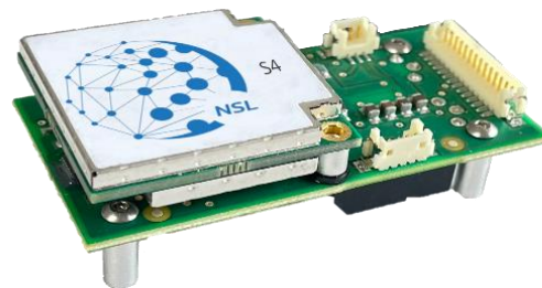
Figure 4 Spaceflight NSL S4 Transceiver for the Iridium network and ground segment (TRL=9).
