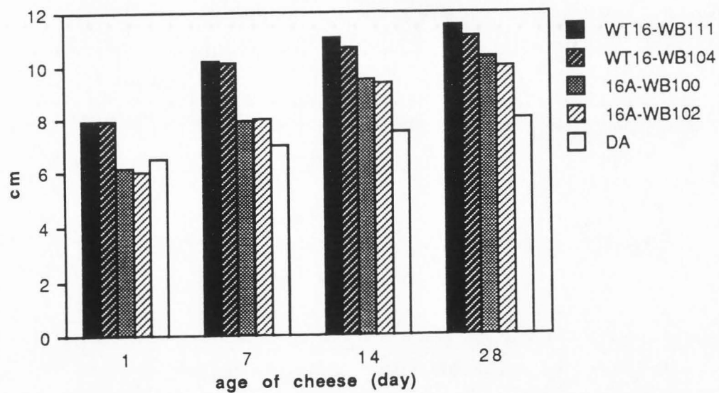
Figure 25. Comparison of meltability of Mozzarella cheeses made with mixed cultures of S. thermophilus and L. bulgaricus (ratio of coccus/rod = 30/70).
