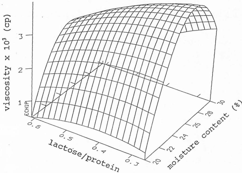
Figure 12. Response surface for viscosity as plotted for moisture content and lactose/protein ratio with protein content and feed rate fixed at mid-point values.
