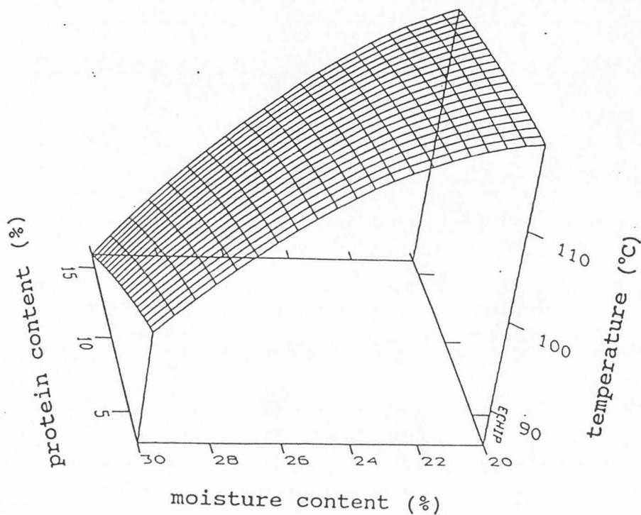
Figure 5. Response surface for product temperature as plotted for moisture content and protein content with lactose/protein ratio and feed rate fixed at mid-point values.
