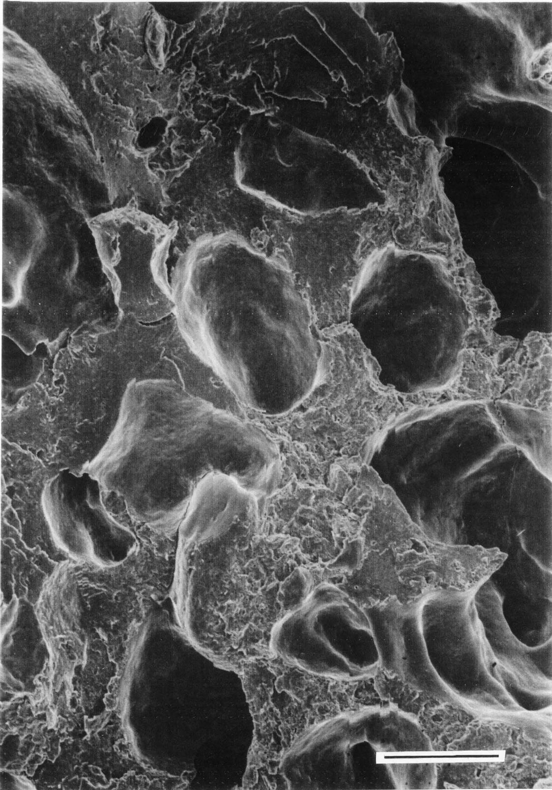
Figure 21. Scanning electron micrograph of the extrudate produced with maximum values for all four control variables (run 3, Table 4). The micron bar has length equal to 30  $\mu\text{m}$ .
