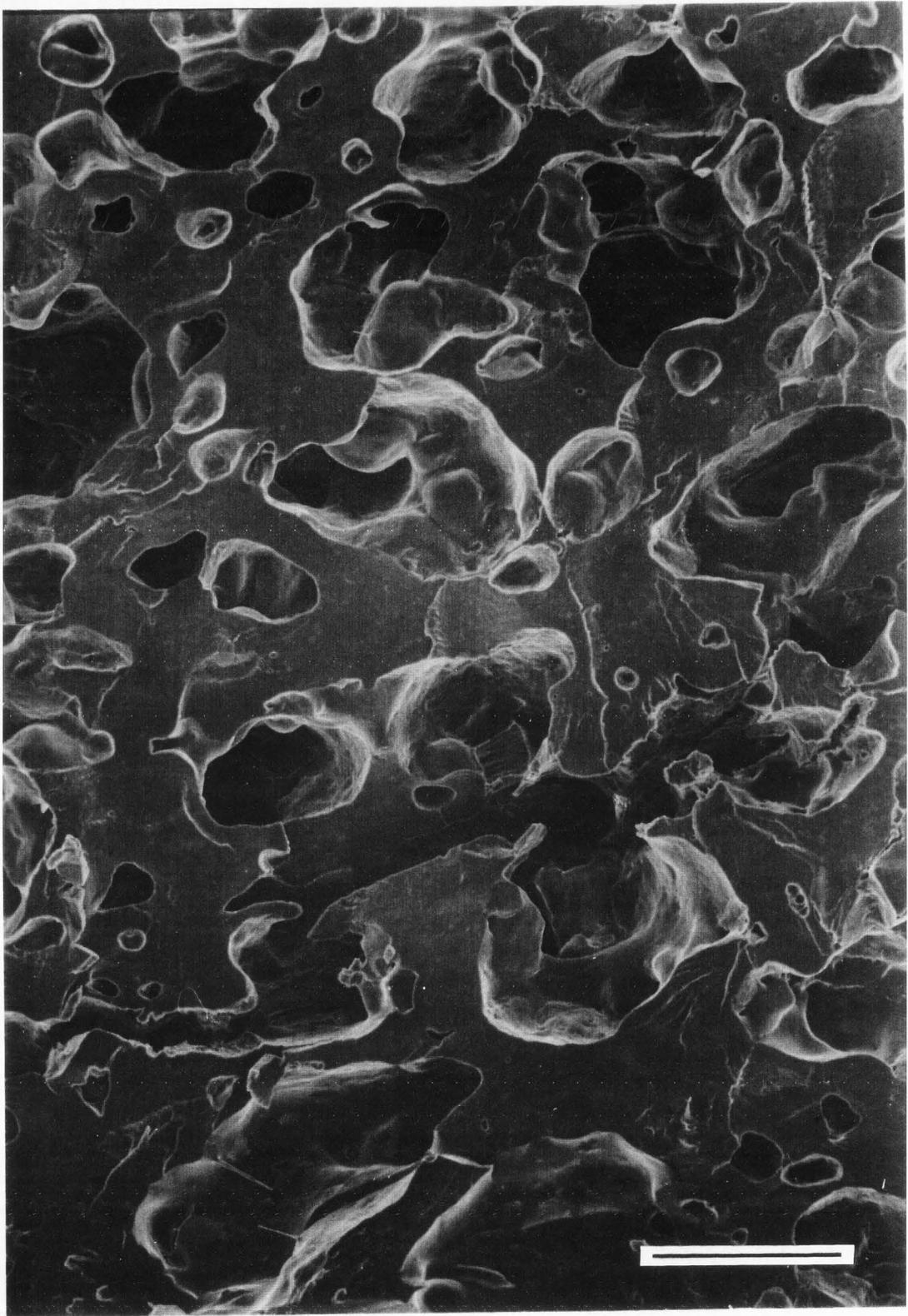
Figure 22. Scanning electron micrograph of the extrudate produced with center point values for all four control variables (run 1, Table 4). The micron bar has length equal to 30  $\mu\text{m}$ .
