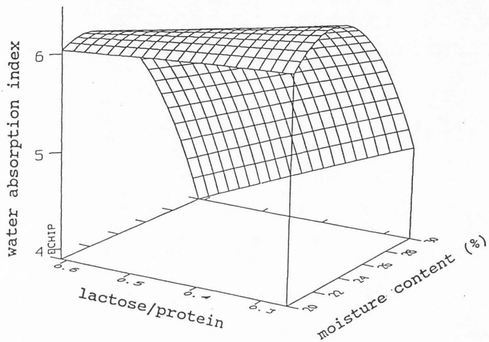
Figure 16. Response surface for water absorption index as plotted for moisture content and lactose/protein ratio with protein content and feed rate fixed at mid-point values.
