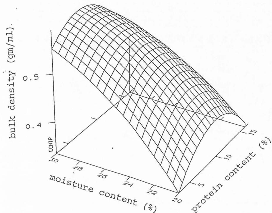
Figure 7. Response surface for bulk density as plotted for moisture content and protein content with lactose/protein ratio and feed rate fixed at mid-point values.
