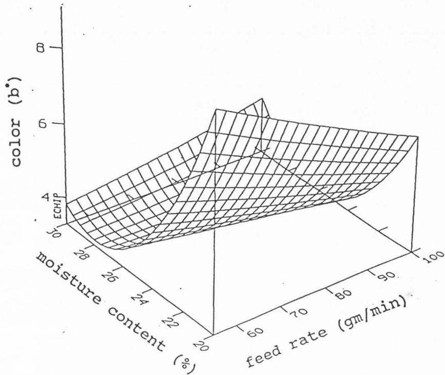
Figure 9. Response surface for color as plotted for moisture content and feed rate with protein content and lactose/protein ratio fixed at mid-point values.
