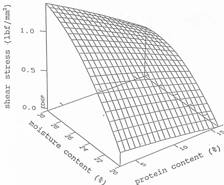
Figure 10. Response surface for shear stress as plotted for moisture content and protein content with lactose/protein ratio and feed rate fixed at mid-point values.
