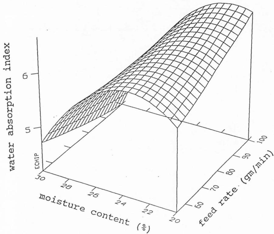
Figure 14. Response surface for water absorption index as plotted for moisture content and feed rate with protein content and lactose/protein ratio fixed at mid-point values.
