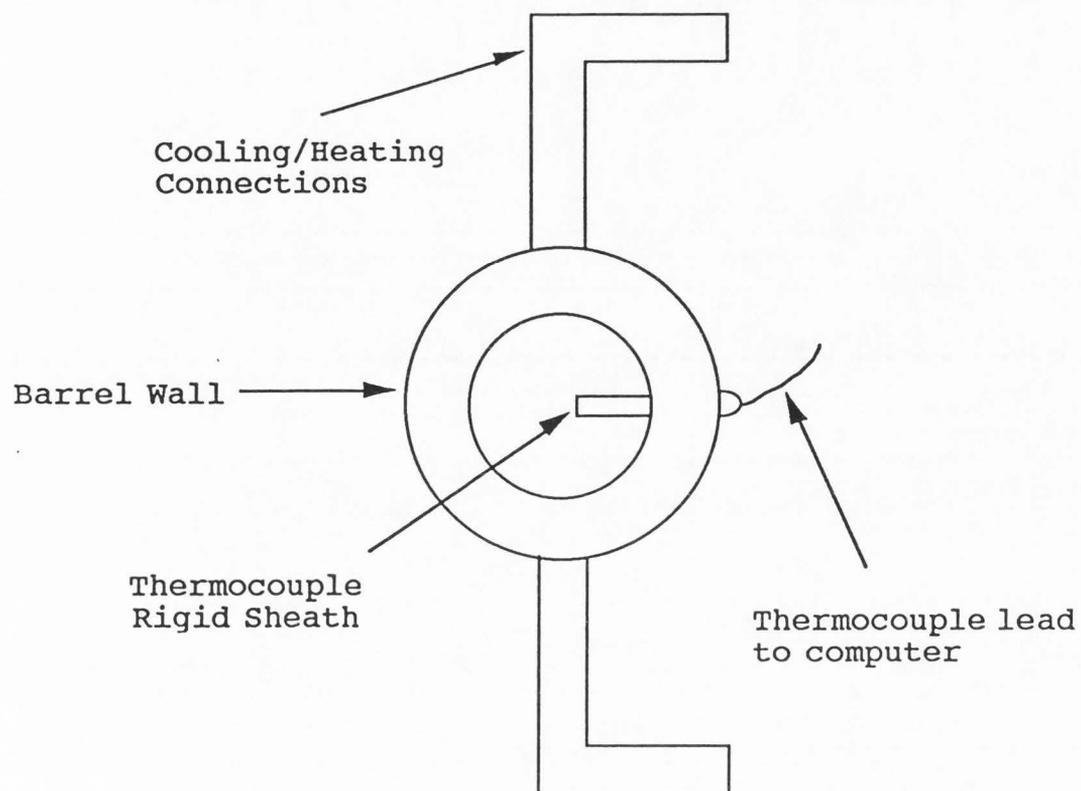
Figure 2. Barrel spacer equipped with thermocouple.
