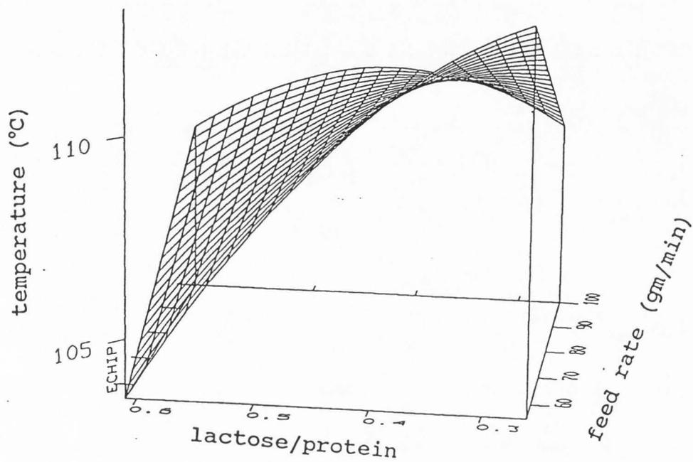
Figure 6. Response surface for product temperature as plotted for lactose/protein ratio and feed rate with moisture content and protein content fixed at mid-point values.
