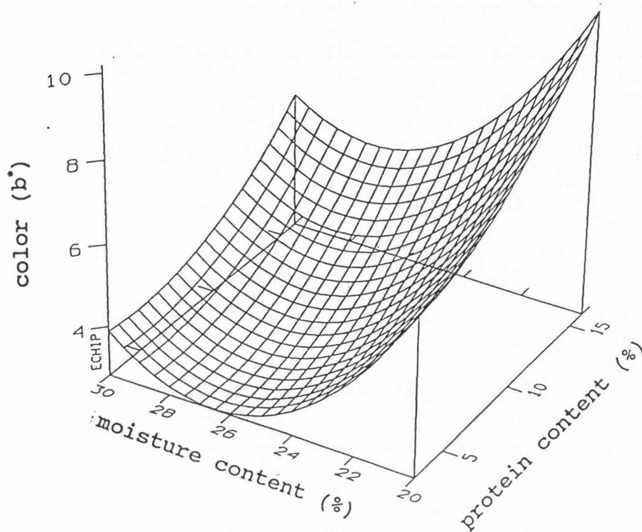
Figure 8. Response surface for color as plotted for moisture content and protein content with lactose/protein ratio and feed rate fixed at mid-point values.
