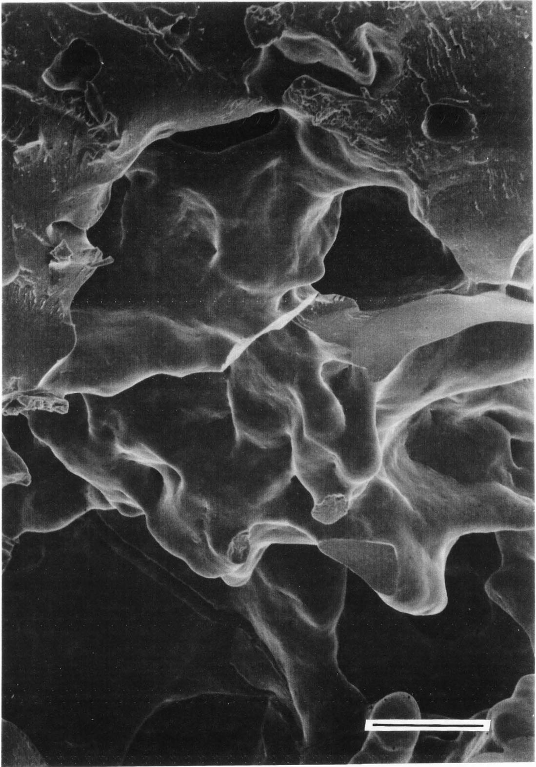
Table 4). The well gelatinized, smooth, continuous matrix of starch was due to maximum gelatinization of starch at 26% moisture content and low protein content and lactose/protein ratio. Air cells were absent, resulting in a dense and compact structure.
