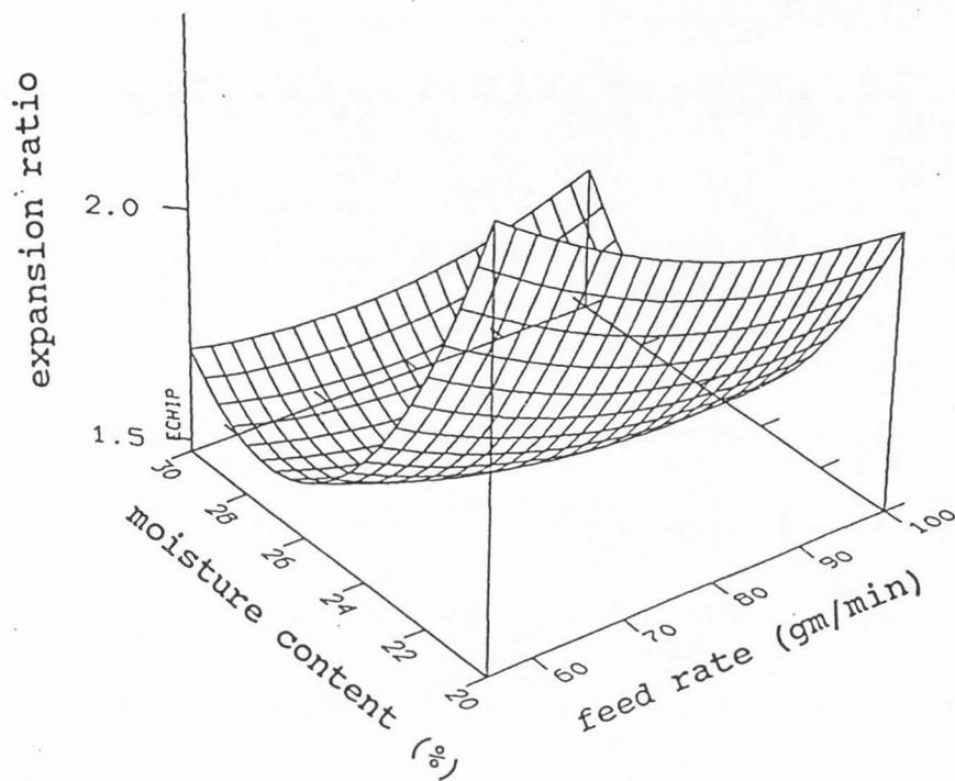
Figure 4. Response surface for expansion ratio as plotted for moisture content and feed rate with protein content and lactose/protein ratio fixed at mid-point values.
