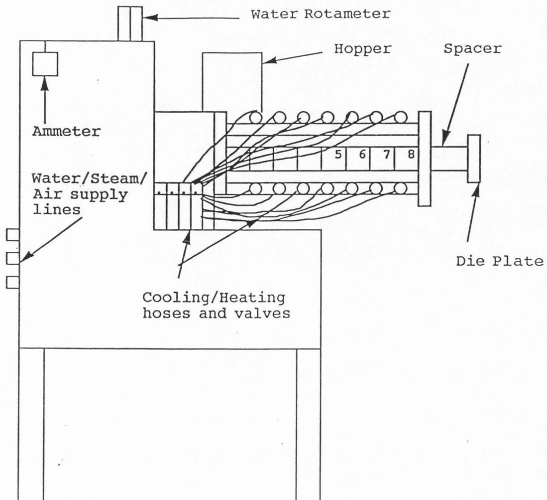
Figure 1. Wenger X-5 single-screw extruder
