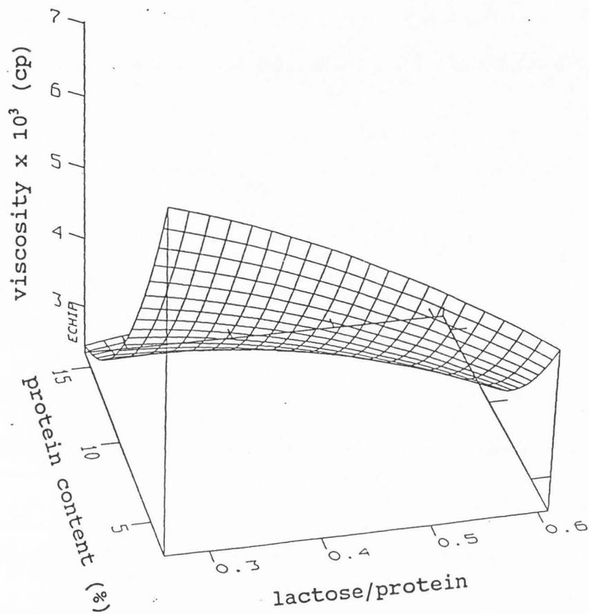
Figure 13. Response surface for viscosity as plotted for protein content and lactose/protein ratio with moisture content and feed rate fixed at mid-point values.
