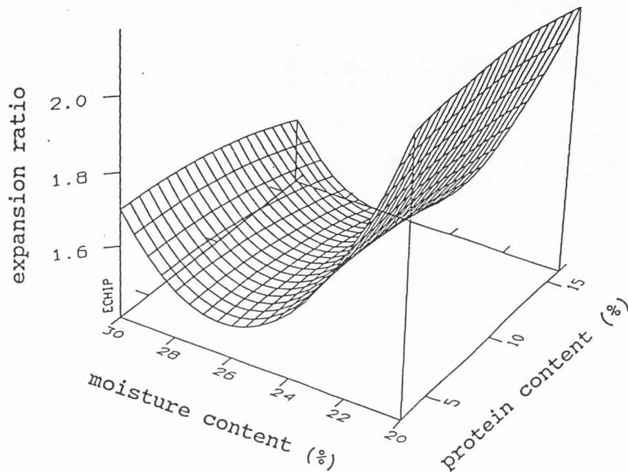
Figure 3. Response surface for expansion ratio as plotted for moisture content and protein content with lactose/protein ratio and feed rate fixed at mid-point values.
