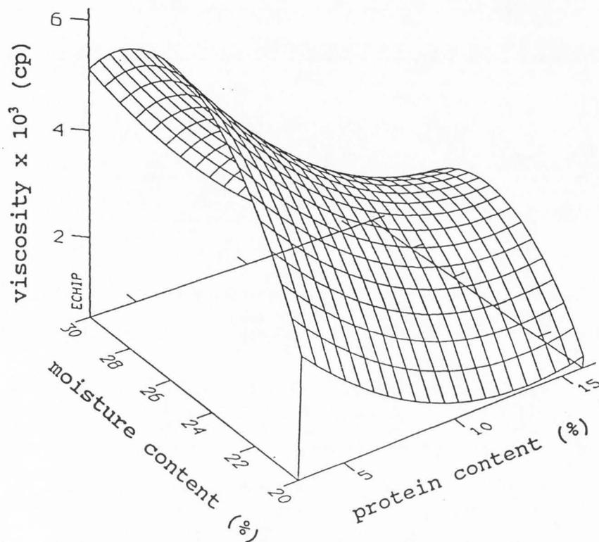
Figure 11. Response surface for viscosity as plotted for moisture content and protein content with lactose/protein ratio and feed rate fixed at mid-point values.
