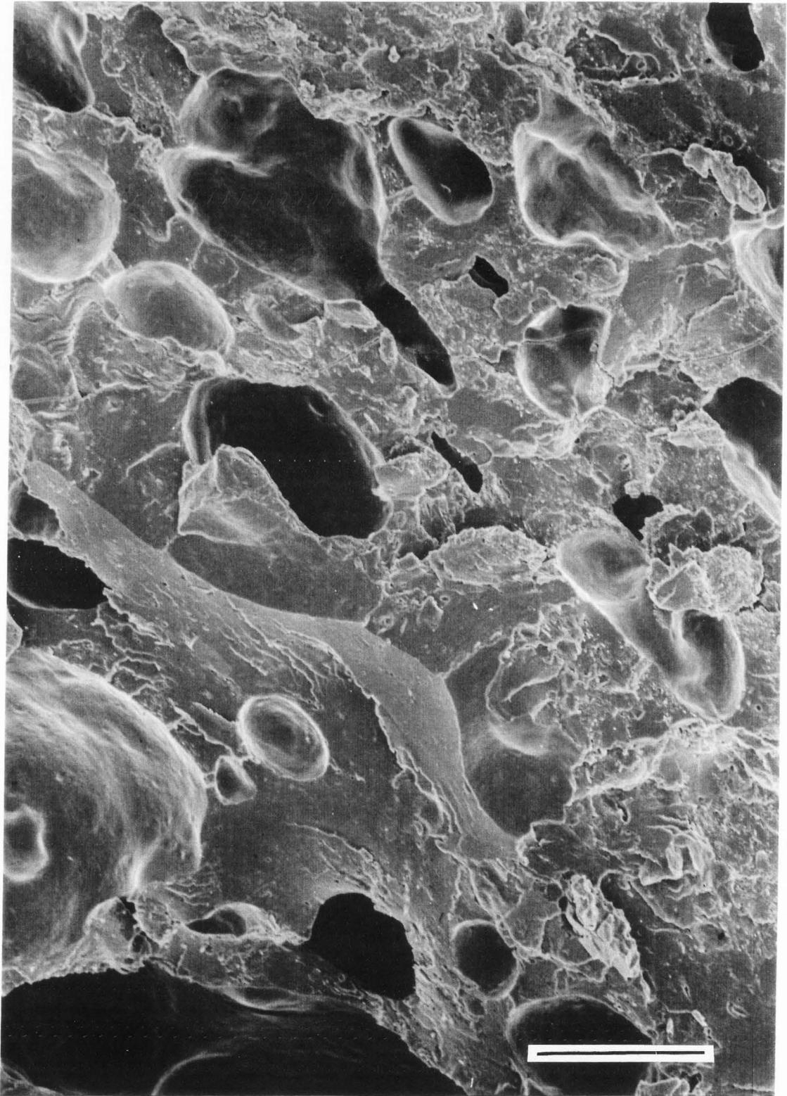
Figure 18. Scanning electron micrograph of the extrudate produced with minimum moisture content (run 5, Table 4). The micron bar has length equal to 30  $\mu\text{m}$ .
