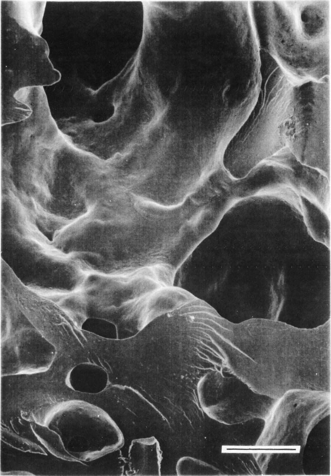
Figure 20. Scanning electron micrograph of the extrudate produced with maximum feed rate (run 29, Table 4). The micron bar has length equal to 30  $\mu\text{m}$ .
