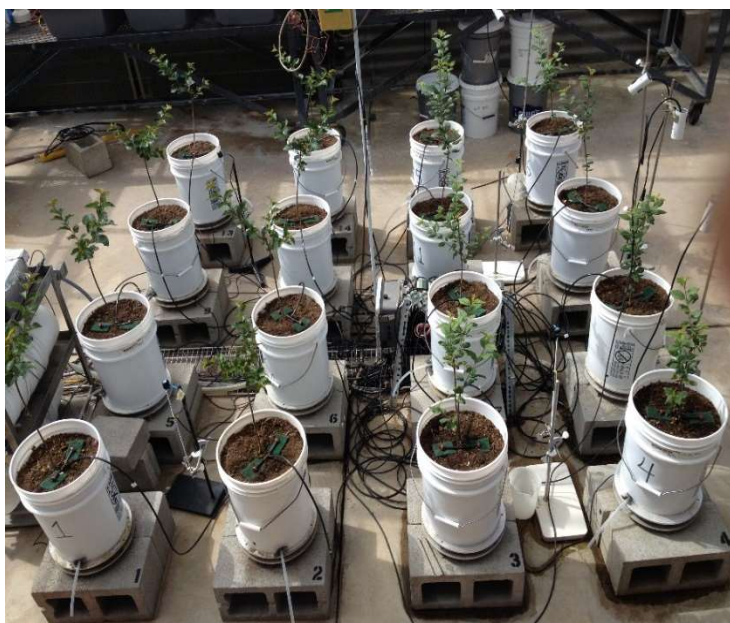
Fig. 2.3.1. Gisela 5 and Gisela 12 rootstocks on weighing lysimeters.
