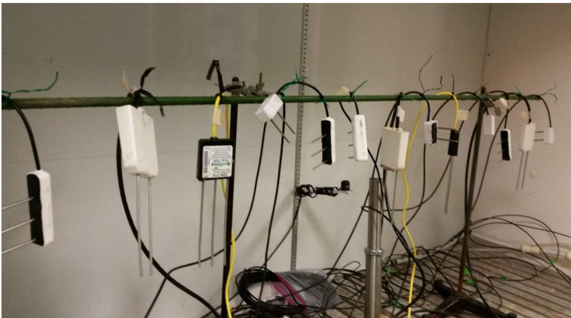
Fig. A.2.1. Temperature sensitivity of five types of electromagnetic soil moisture sensors. All sensors were suspended the air in a dark controlled environment chamber with large diurnal temperature gradients to determine electronics temperature sensitivity.
