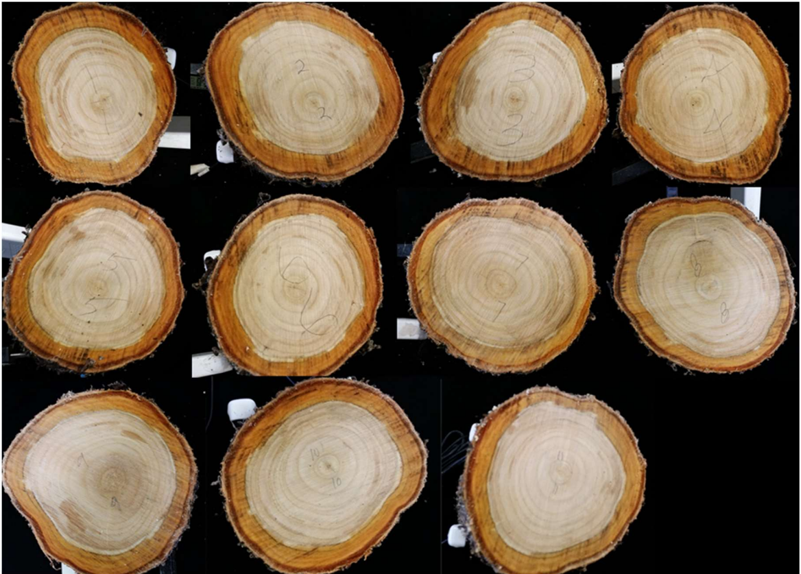
Fig. 3.3.12. Sapwood and heartwood ratios for all excised peach trunk sections. Sapwood was comprised of the outer four or five annular rings and was about 3 cm thick.
