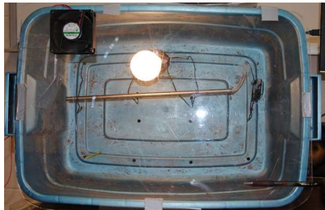
Fig. F.2.5. Simulated growth chamber used to test programs and real-time interfaces.
