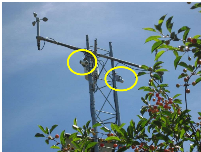
Fig. 4.3.6. Infrared radiometers mounted near the top of a weather station tower. Generally, one sensor faced east and one faced west.
