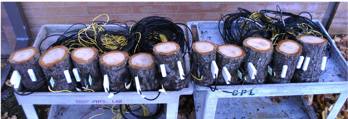
Fig. 3.3.11. Excised peach trunk sections with installed electromagnetic sensors. A total of 22 sensors were installed in 11 Peach trees.
