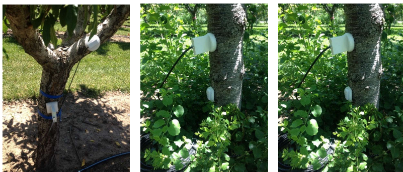
Fig. 3.3.5. Electromagnetic soil moisture sensors installed in fruit trees 2015. Sensors were inserted in Peach trunks and scaffold branches (left), Tart Cherry trunks (left) and Apple trunks (right) .
