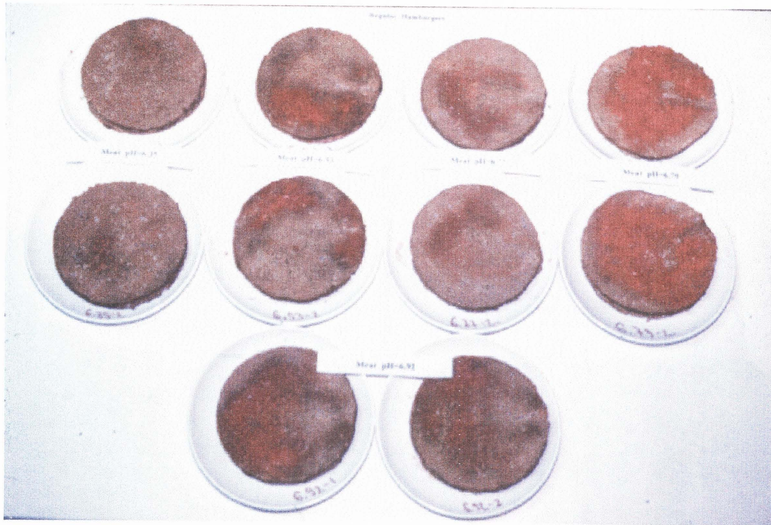
Fig. 15 -- Inside surface of lean hamburgers of pH=6.35-6.92 (from left to right) cooked to 71°C internal temperature.
