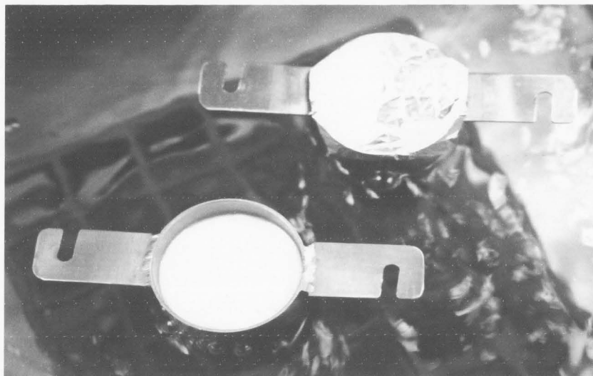
Figure 5.3. Sample cups containing cheese temper in a water bath. Slotted wings were used to secure the cups to the sample cup holder. It was determined that cheese plugs, rather than ground cheese, provided more homogeneous melted cheese texture and therefore more consistent results than did ground cheese samples. Aluminum cover reduced evaporation.
