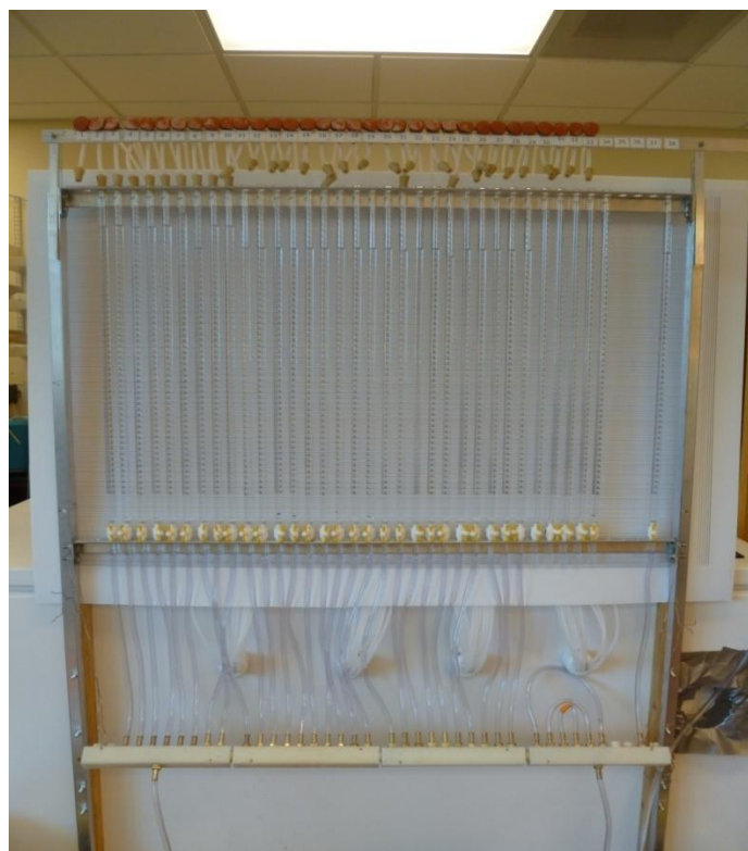
Fig. 3.2 Image of 36 burette biogas monitoring system. Each burette has septum located at top to remove biogas produced.
