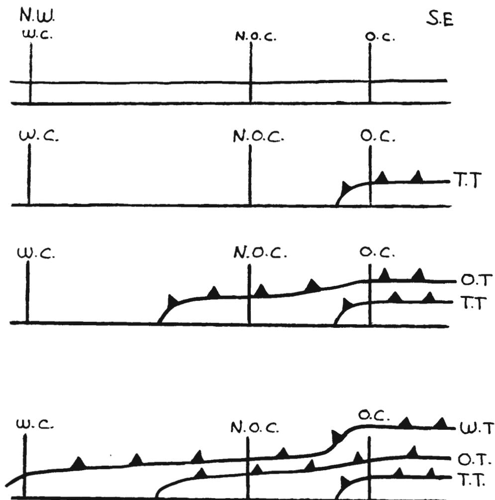
Fig. 25 Hangingwall sequence diagrams showing a simplified longitudinal development (NW-SE) of the Willard "thrust complex." Horizontal scale is 1:100,000. N.W.-Northwest, S.E.-Southeast, W.C.-Willard Canyon, N.O.C.-North Ogden Canyon, O.C.-Ogden Canyon, T.T.-Taylor Thrust, O.T.-Ogden Thrust, W.T.-Willard Thrust.
