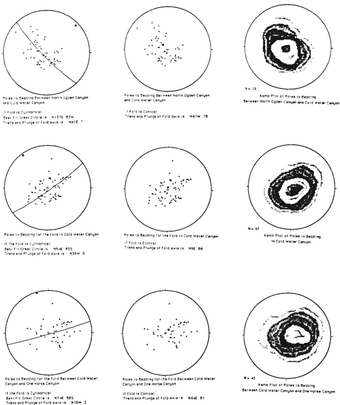
Fig. 15 Stereonet plots of orientations of poles to bedding at the Cold Water Canyon field area.
