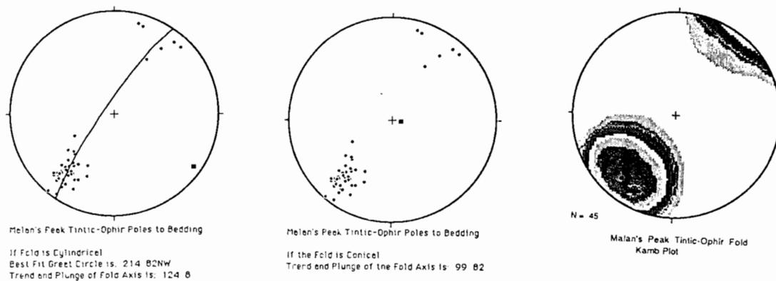
Fig. 18 Stereonet plots of orientations of poles to bedding around the limb of the basement-cored monocline at Malans Peak. Field mapping indicates the fold to be cylindrical.
