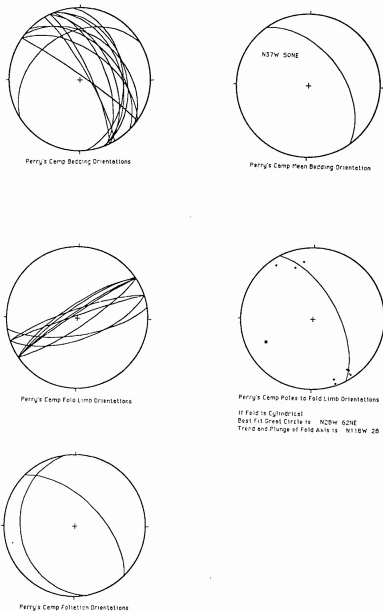
Fig. 21 Stereonet plots of orientations of deformation structures at the Perry's Camp field area. See Appendix B for the number of data points used. The mean bedding orientation was calculated from all bedding data.
