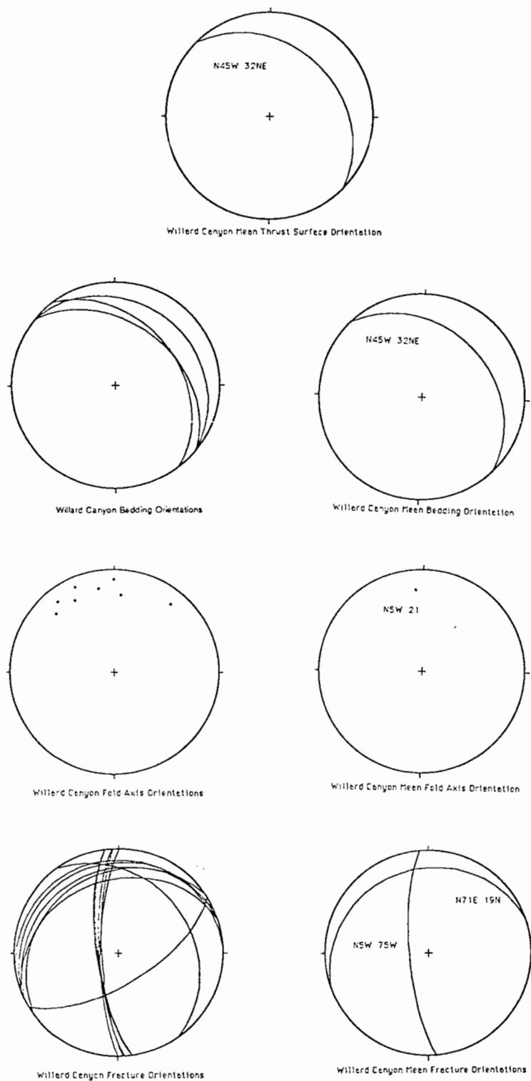
Fig. 9 Stereonet plots of orientations of deformation structures at the Willard Canyon field area. See Appendix B for the number of data points used. Plotted data was visually grouped and means were calculated and plotted from resulting groups.
