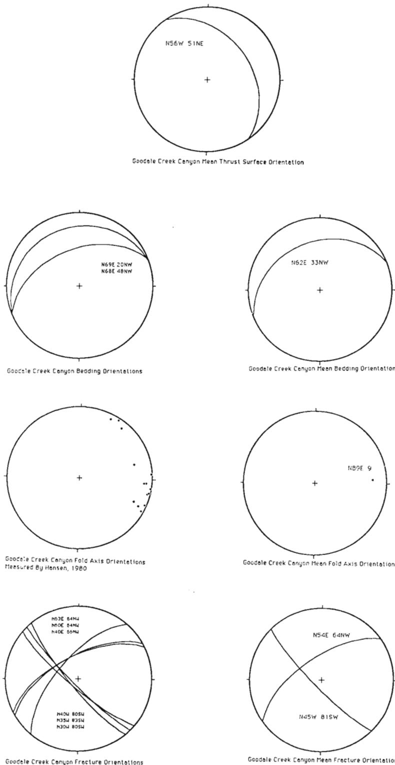
Fig. 16 Stereonet plots of orientations of deformation structures at the Goodale Creek Canyon field area. See Appendix B for the number of data points used. Plotted data was visually grouped and means were calculated and plotted from the resulting groups.
