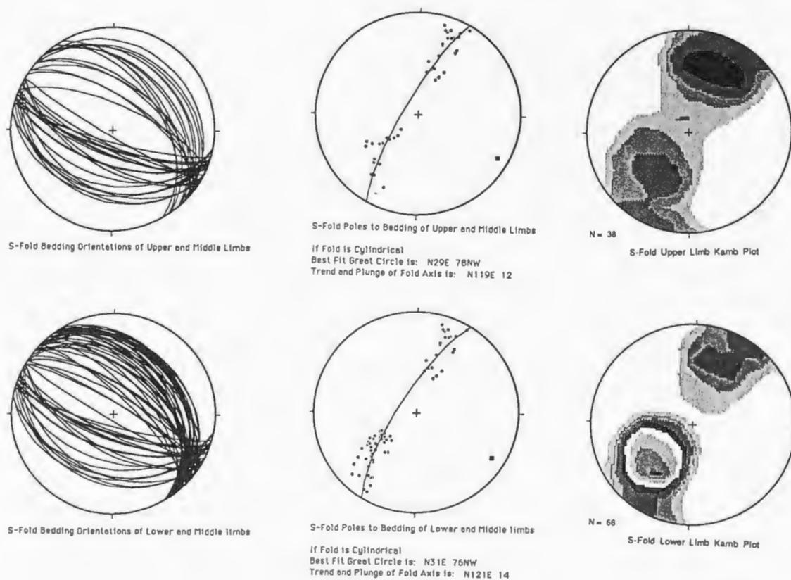
Fig. 20 Stereonet plots of orientations of bedding for the upper, middle, and lower limbs of the "S" Fold. See Appendix B for the number of data point used.
