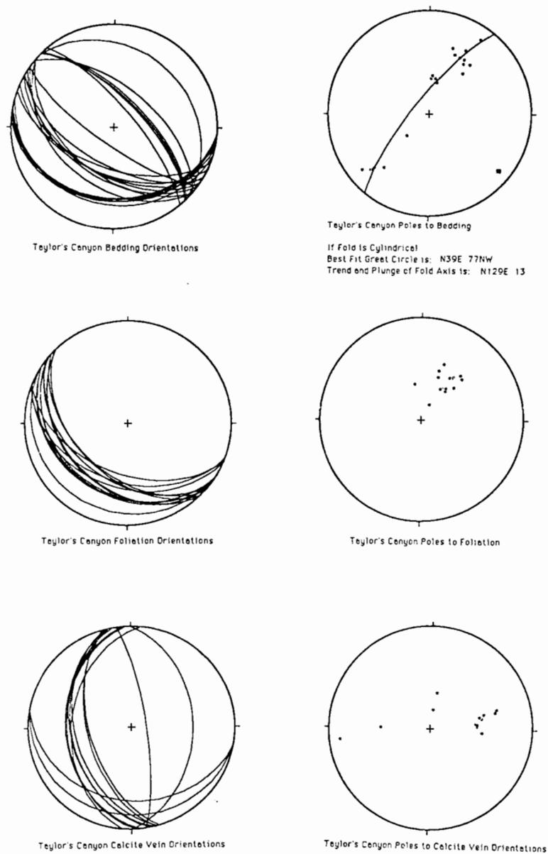
Fig. 19 Stereonet plots of orientations of deformation structures at the Taylor Canyon field area. See Appendix B for the number of data points used.
