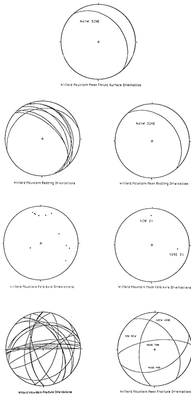
Fig. 10 Stereonet plots of orientations of deformation structures at the Willard Mountain field area. See Appendix B for the number of data points used. Plotted data was visually grouped and means were calculated and plotted from resulting groups.
