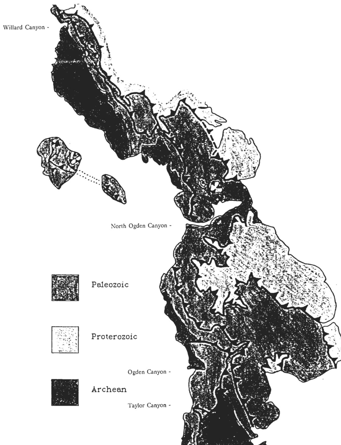
Fig. 3 Generalized geologic map showing footwall (Paleozoic) and hanging wall (Proterozoic) geology of the Willard thrust complex between Willard and Ogden canyons (modified from Schirmer, 1988). Teeth are located on the hanging wall of the thrusts.
