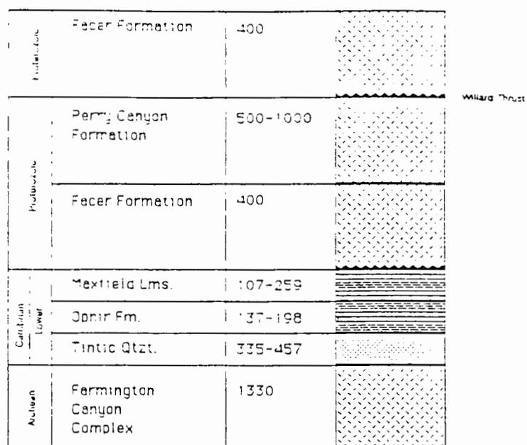
Fig. 28 Generalized stratigraphic column of Willard Canyon. Unit thicknesses are reported in meters from Hintze (1988).
