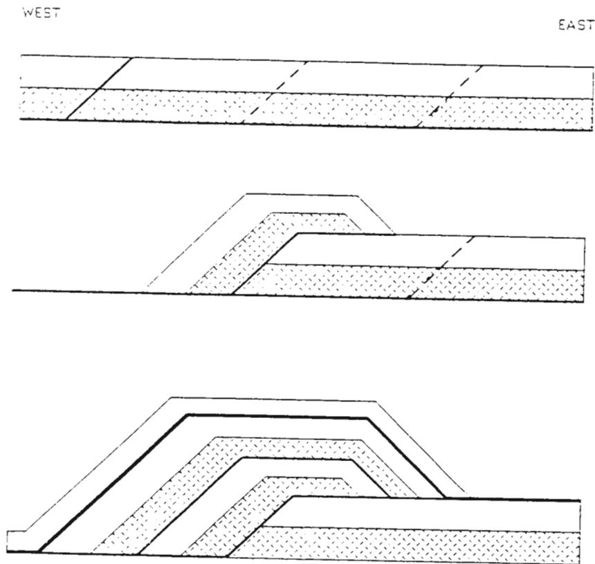
Fig. 2 Schematic diagrams (modified from Boyer and Elliot, 1982) showing developmental geometry of a "classic" foreland-dipping duplex. Older thrust sheets are carried piggyback on younger thrust sheets as the footwall progressively fails (ramping upsection) from left to right.
