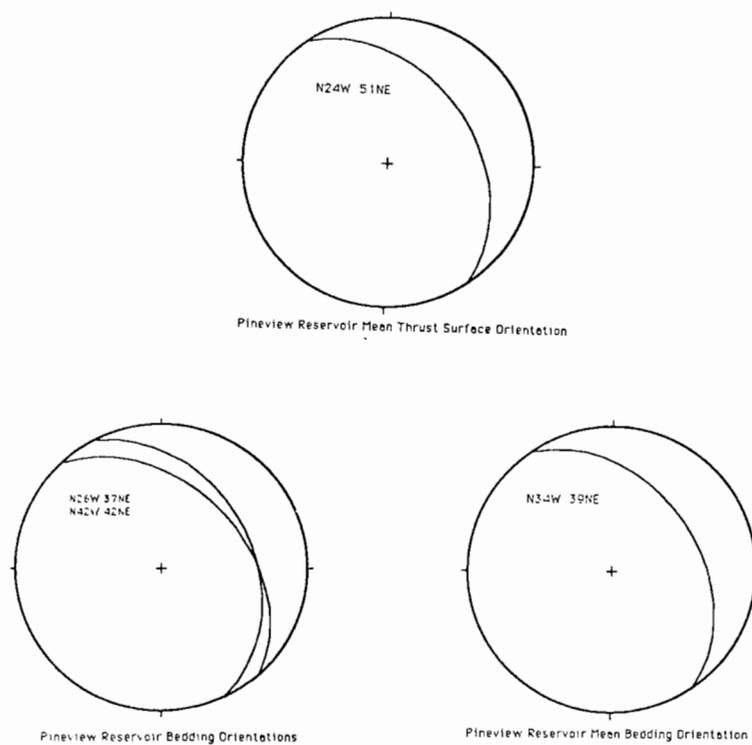
Fig. 17 Stereonet plots of orientations of deformation structures at the Pineview Reservoir field area. See Appendix B for the number of data points used. Plotted data was visually grouped and means were calculated and plotted from resulting groups.
