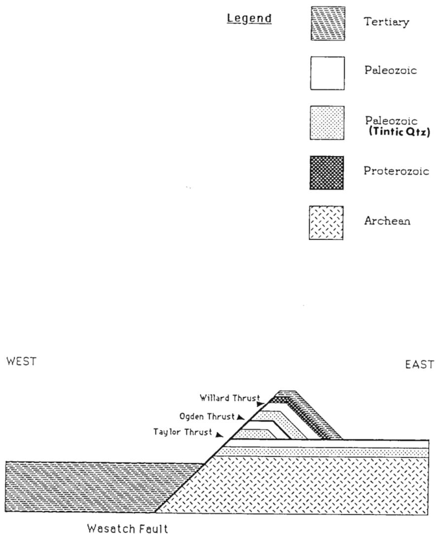
Fig. 5 Schematic diagram showing a generalized conception of the east dipping Willard thrust complex and superimposed Wasatch "normal" fault. The cross-section is oriented west-east and is representative of the geology on the north side of Ogden Canyon.
