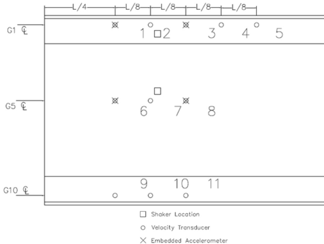
**Figure 25: Sensor Layout during the First Shaker Test**
