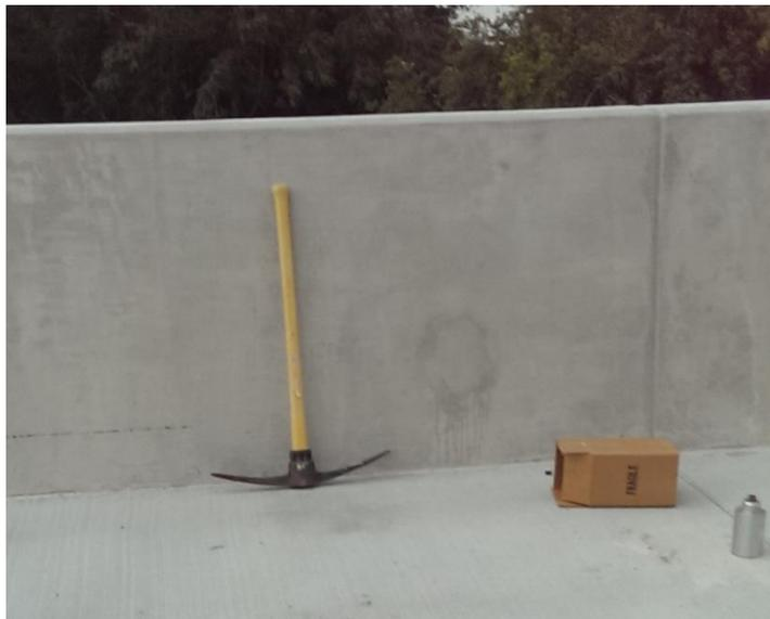
**Figure 19: Pickaxe used to Excite the Bridge during Impact Test**
