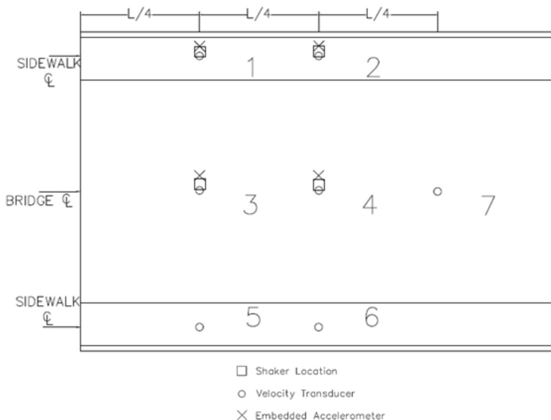
**Figure 20: Sensor Layout during the Impact Test**
