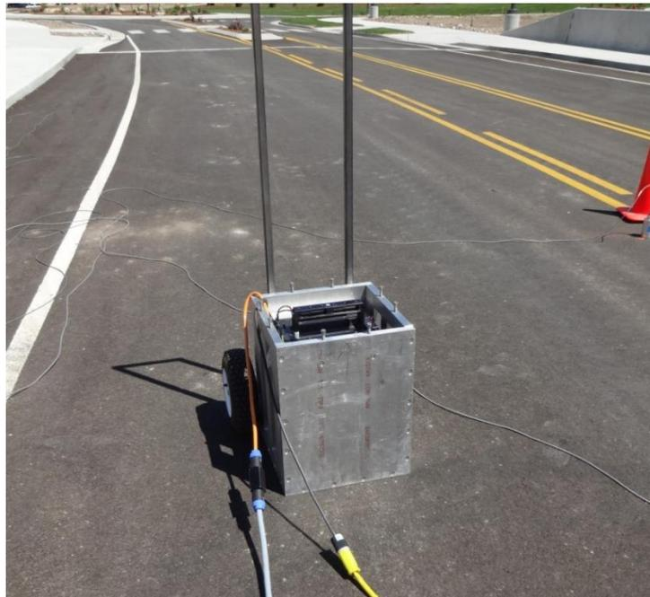
**Figure 17: APS Shaker during First Shaker Test**
