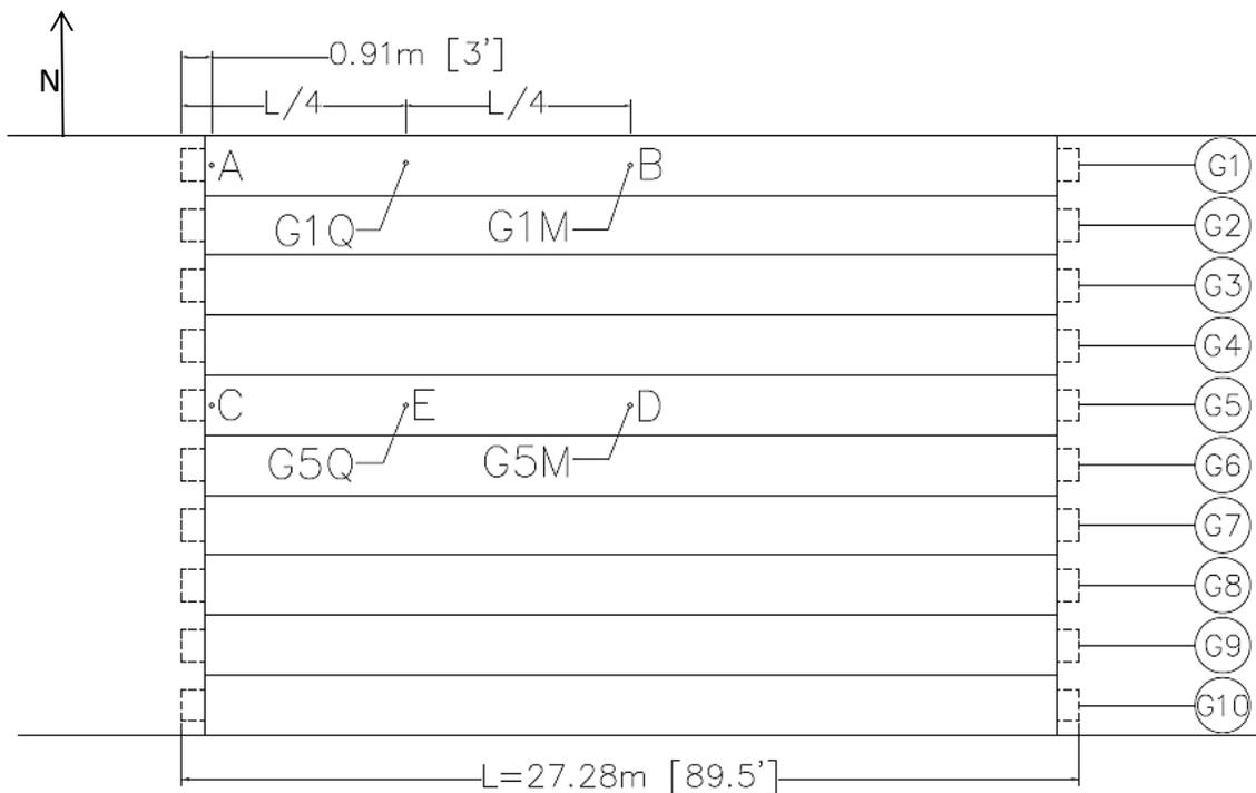
**Figure 8: Instrument Layout Plan View**
