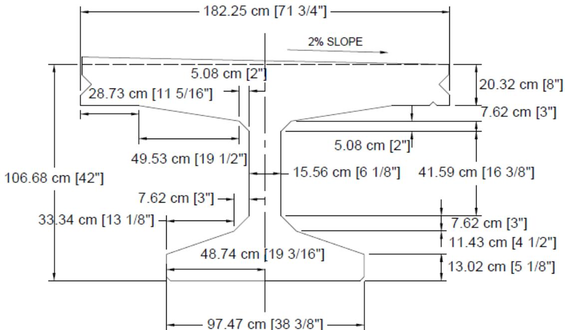
**Figure 7: Construction Dimensions of a Typical Girder (Ethan Pickett, personal communication, Feb. 21, 2017)**
