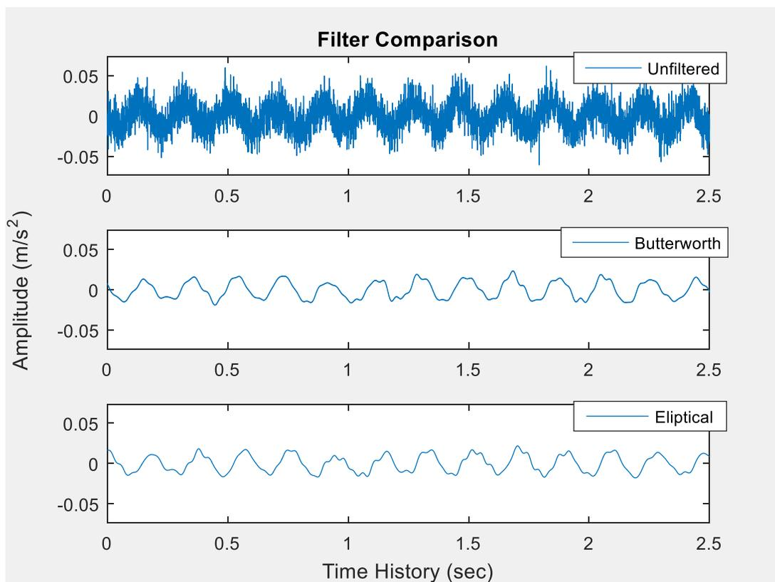
**Figure 31: A Comparison of the Filtered Signals**
