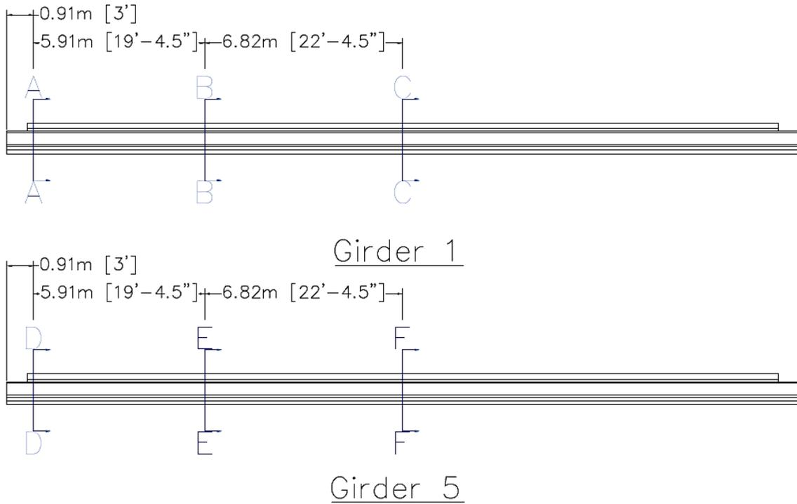
**Figure 9: Girder 1 and Girder 5 Section Cut Locations**
