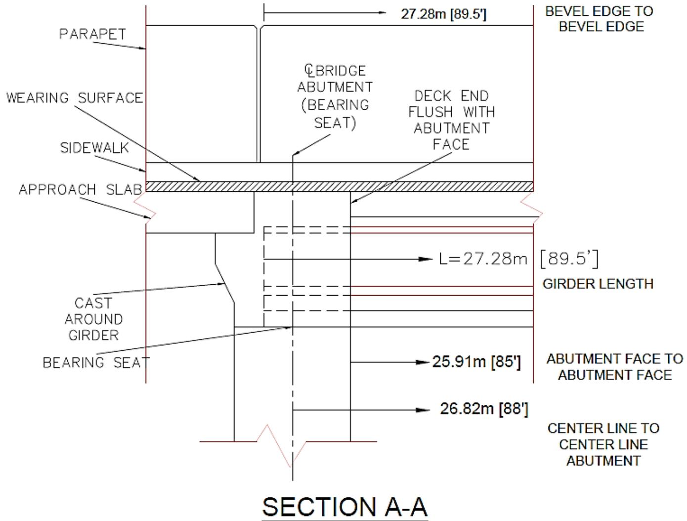
Figure 5: End Section of the Bridge, Section AA from Figure 4
