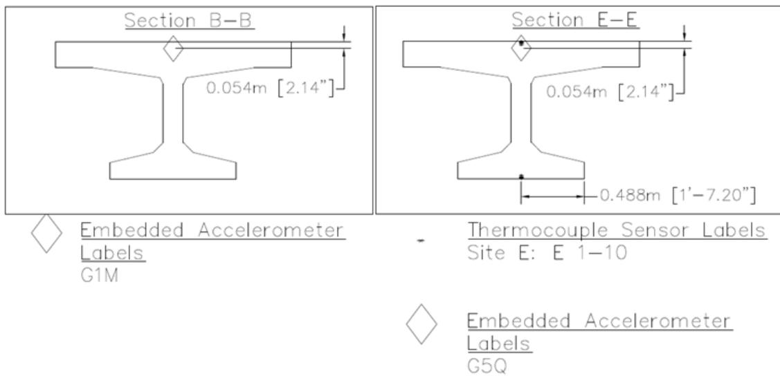
**Figure 12: Instrument Layout Section B-B and E-E**
