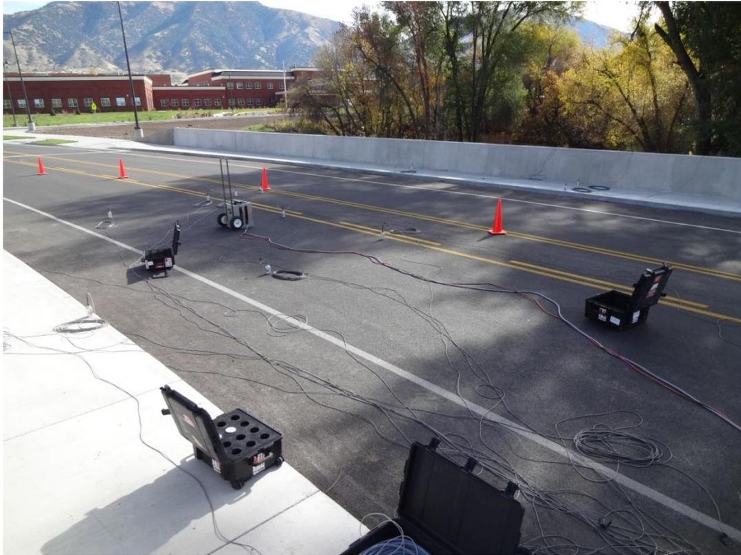
**Figure 27: Sensors and the Shaker during the Second Shaker Test**
