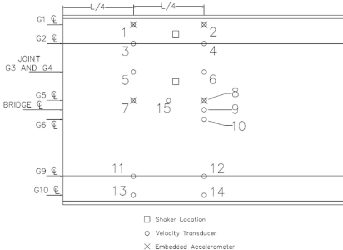
**Figure 26: Sensor Layout during the Second Shaker Test**
