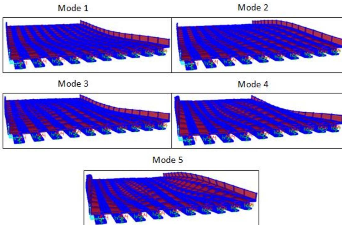
**Figure 38: Analytical Mode Shapes of Corrected Model**
