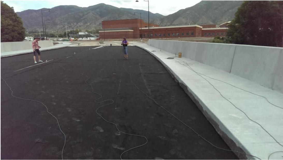
**Figure 18: Preparing Sensors for the Impact Test**
