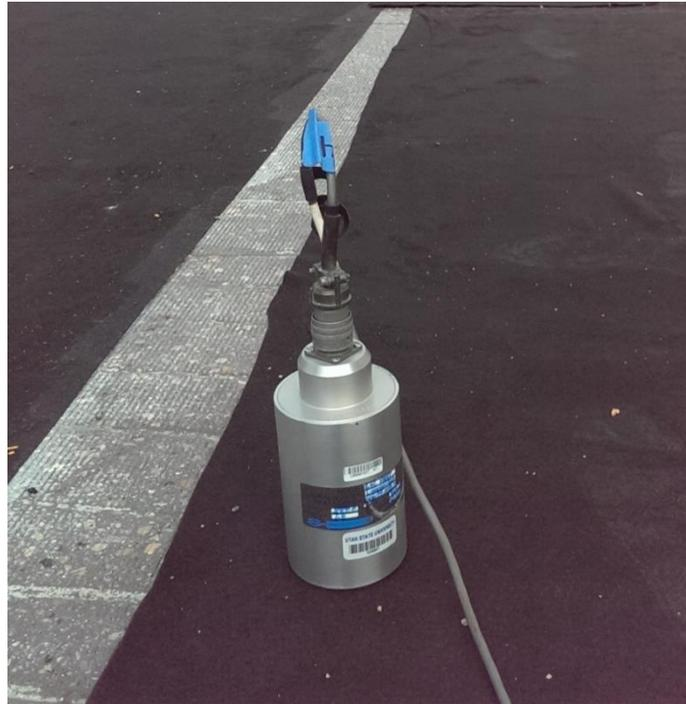
**Figure 16: Velocity Transducer on the Bridge prior to Asphalt Installation**
