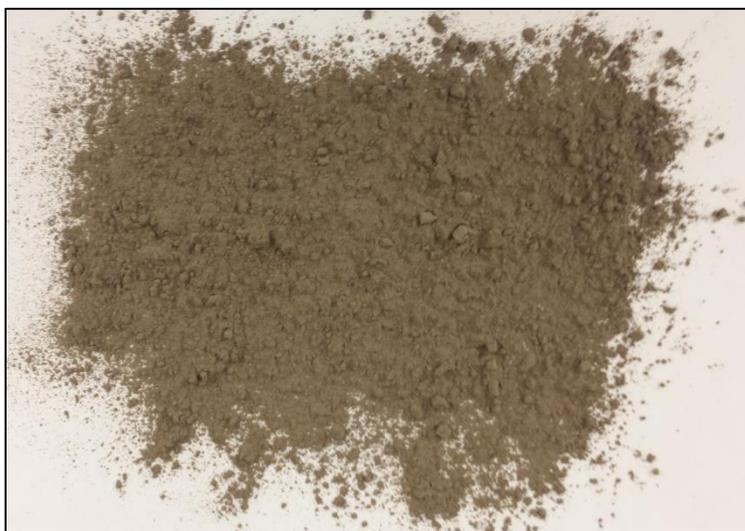
Figure B.3. Powdered expanded shale used as a coagulant
