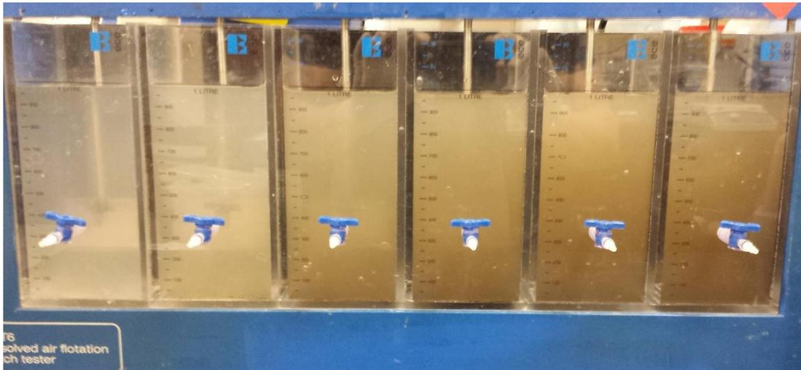
Figure B.5. Jar test demonstrating coagulation-flocculation ineffectiveness of expanded shale in kaolin-humic acid media. Expanded shale concentration left to right 0, 0.5, 1, 2, 5, 10 g/L. (Data from this not presented in this document, figure serves as a visual example of unsuccessful coagulation-flocculation).
