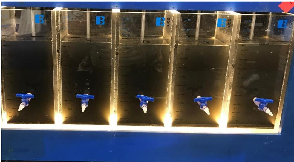
Figure B.5. Jar test demonstrating coagulation-flocculation ineffectiveness of expanded shale in resuspended sludge media. Expanded shale concentration left to right 0, 0.5, 1, 2, 5, 10 g/L. (Data from this not presented in this document, figure serves as a visual example of unsuccessful coagulation-flocculation).
