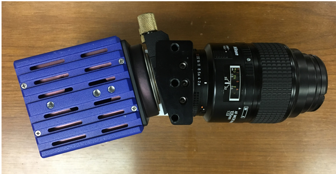
Fig. 3.3: A Camera and lens attached to a scheinpflug adapter. This adapter allows the camera to move relative to the lens.
