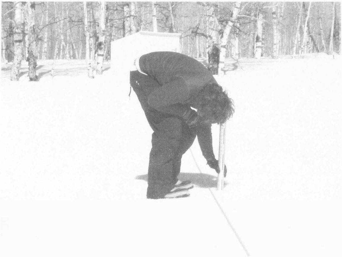
Fig. 3.3 Measurement of snow water equivalent with standard snow tube.
