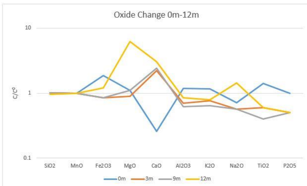
Figure 22. Normalization of major elements from 0 to 12 meters for Fault F1. Major elements normalized to protolith.
