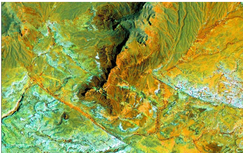
Figure 12. False color NAIP imagery that was used to identify possible faults before field work.
