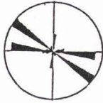
GRIDPTS 1,2,3,15 (Outcrop Fractures) N-309:120-130-32%, 90-100-28%
