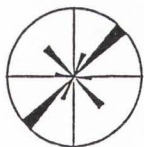
TRAVERSE PT F (Outcrop Fractures) N=49:40-50-45%, 130-140-27%
