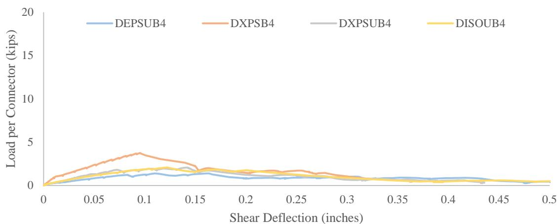
Figure 4-15 Chart of all 4-in. specimens for Connector D
