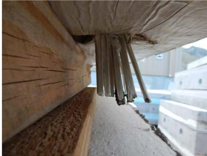
Figure 4-20 Dowel action causing delamination along the width of Connector B
