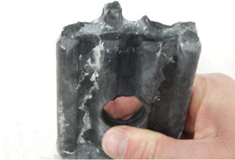
Figure 4-34 Close-up of shear fracture of connector D
