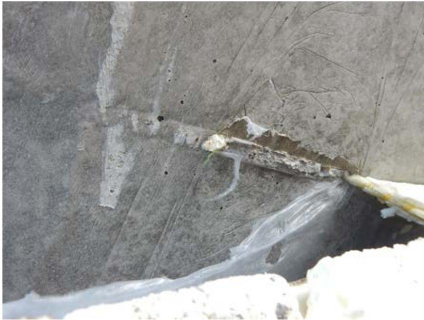
Figure 4-19 Shear fracture failure in unbonded specimen with EPS foam
