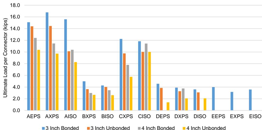
Figure 4-3 Ultimate Load Comparison for All Connectors Individually
