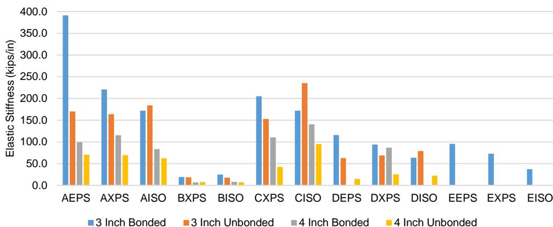
Figure 4-6 Elastic Stiffness Comparison for All Connector
