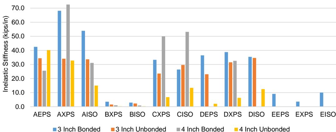
Figure 4-7 Inelastic Stiffness Comparison for All Connector
