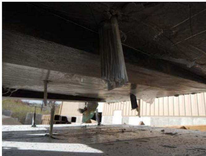
Figure 4-21 Dowel action failure of Connector B
