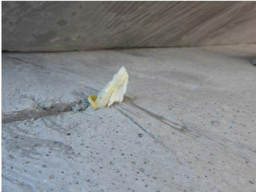
Figure 4-17 Tensile rupture in unbonded specimen with ISO foam
