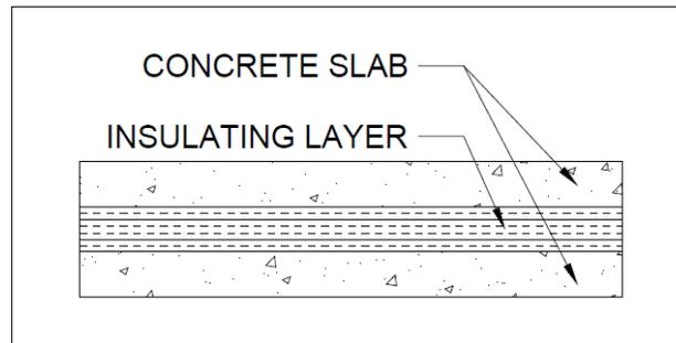
Figure 1-1 Configuration of a Concrete Sandwich Panel
