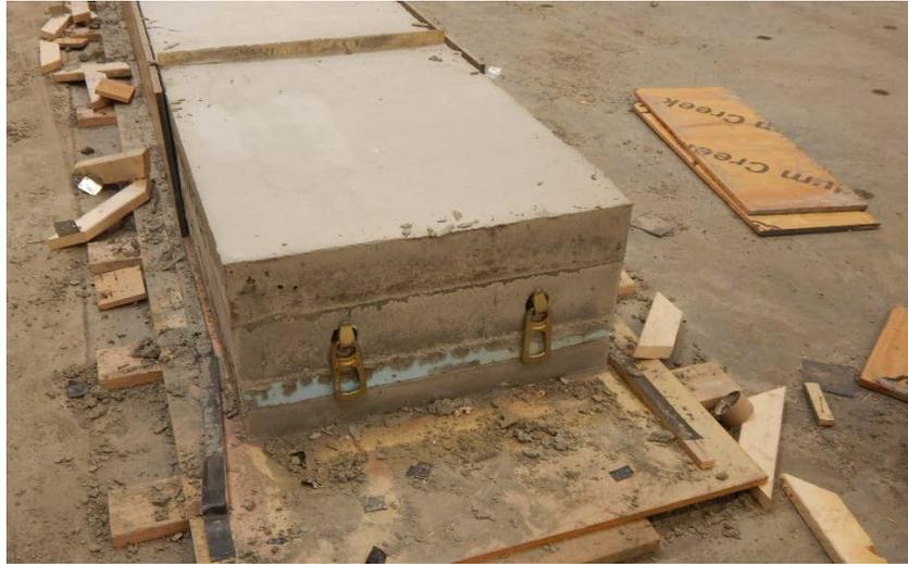
Figure 3-26 Horizontal specimen ready to be lifted.
