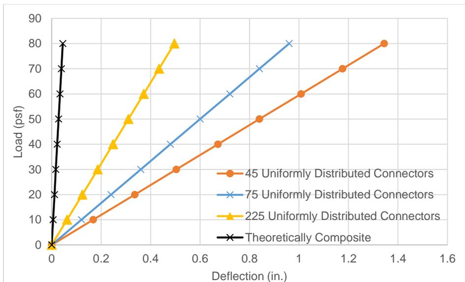
Figure 5-5 Example elastic load versus deformation relationship.
