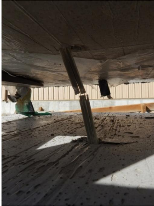
Figure 4-22 Dowel action occurring along the length of Connector B
