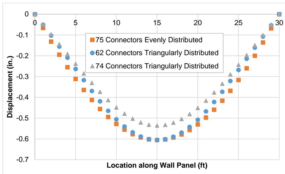
Figure 5-3 Deflection comparison with different connector distributions.
