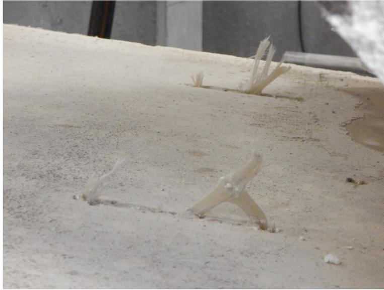
Figure 4-37 Tensile rupture of tension strut in truss.
