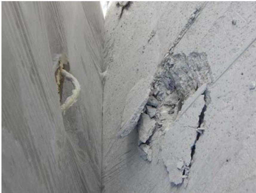
Figure 4-18 Pullout failure in unbonded specimen with ISO foam
