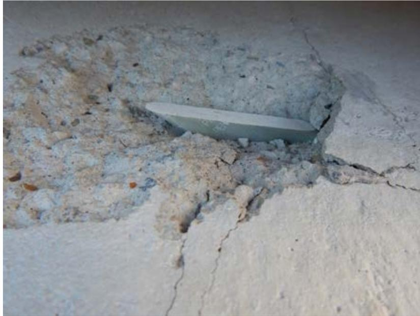
Figure 4-31 Punch through close-up
