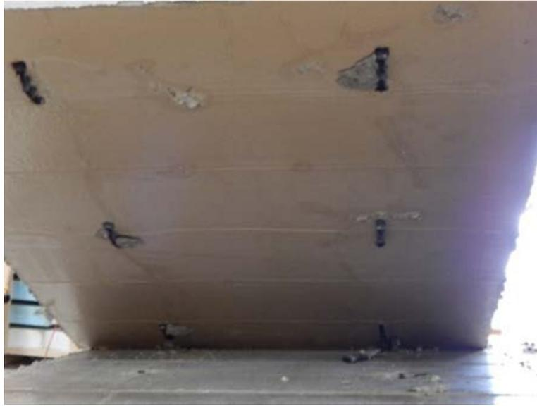
Figure 4-32 Shear fracture of Connector D (full specimen)
