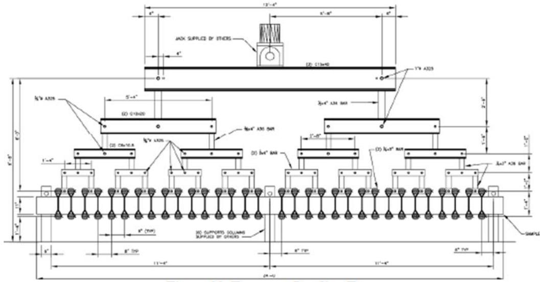
Figure 2-17 Loading pattern applying point loads across unsupported span of panel
