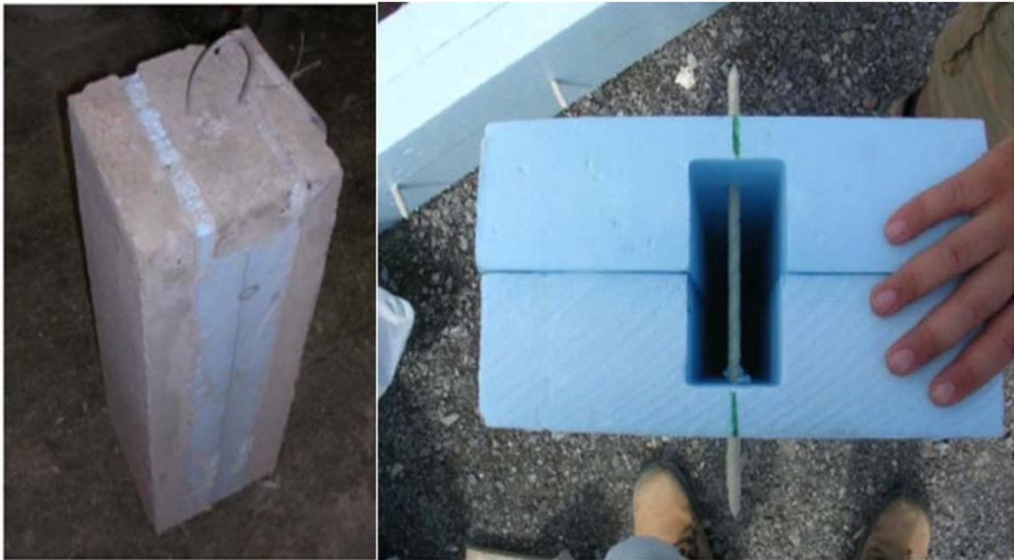
Figure 2-21 Push-off Specimen cured (left) and before concrete poured (right) (Woltman et al. 2013)
