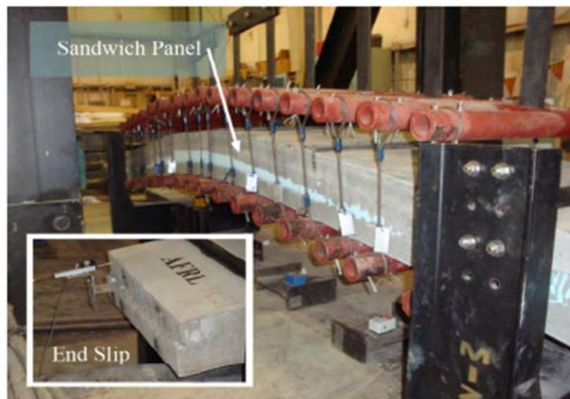
Figure 2-18 Photograph depicting the loading tree and end-slip measurement (Naito et al.
