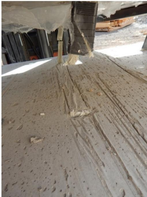
Figure 4-25 Shear fracture of Connector B
