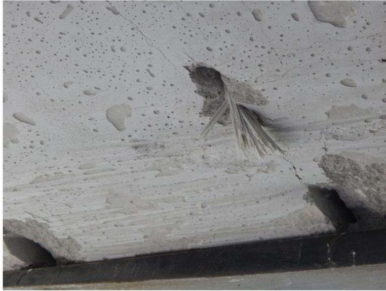
Figure 4-29 Shear fracture and dowel action of Connector C
