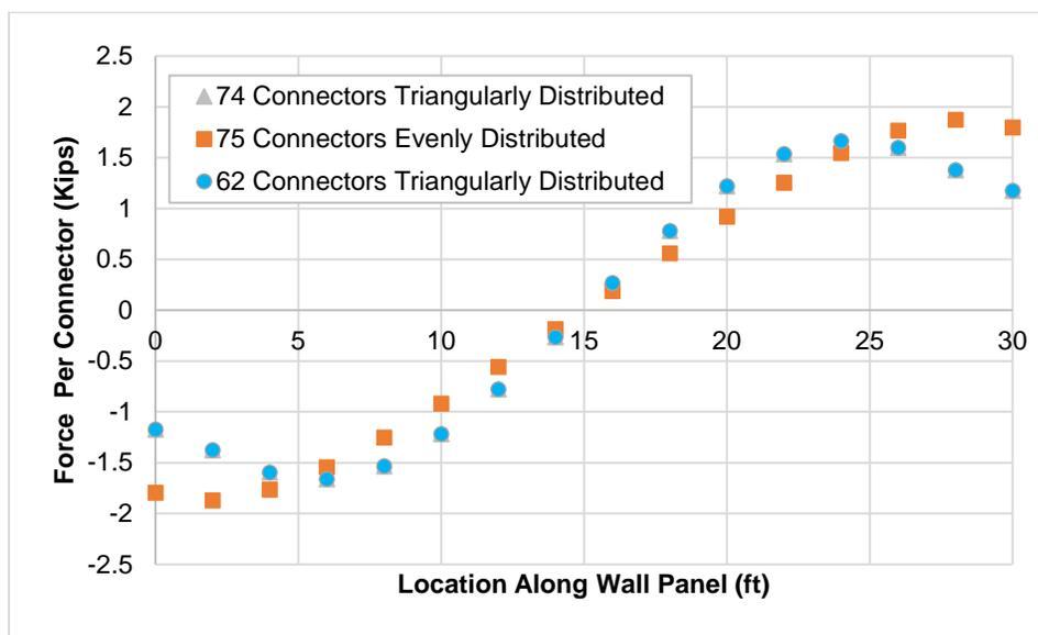
Figure 5-4 Force per connector for different connector distributions.
