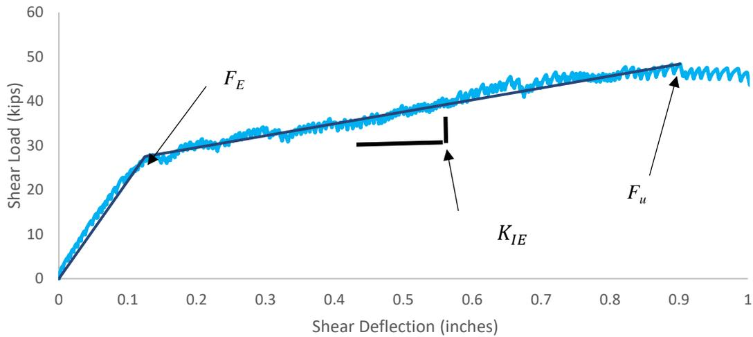
Figure 4-2 Load-Deformation Curve & Visually Identifying the Yield Point
