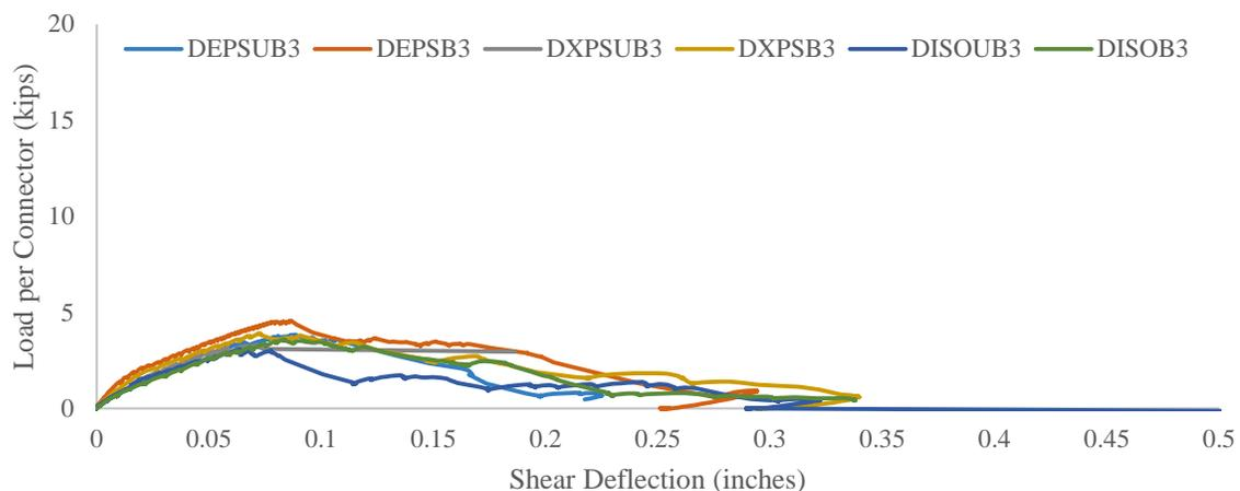
Figure 4-14 Chart of all 3-in. specimens for Connector D
