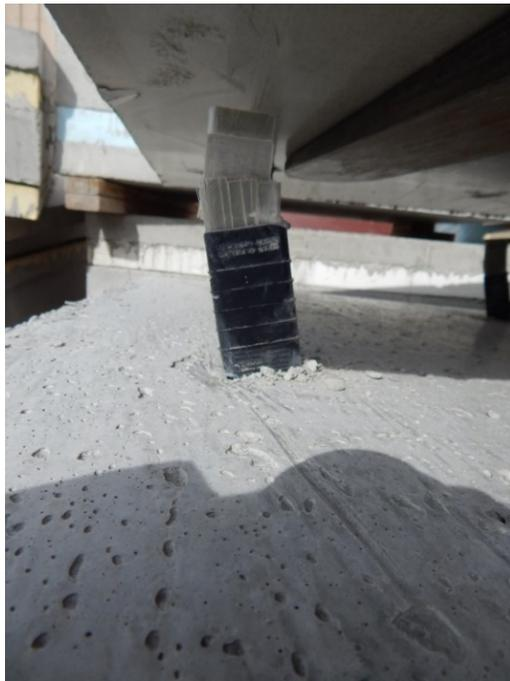
Figure 4-23 Shear fracture observed in Connector B
