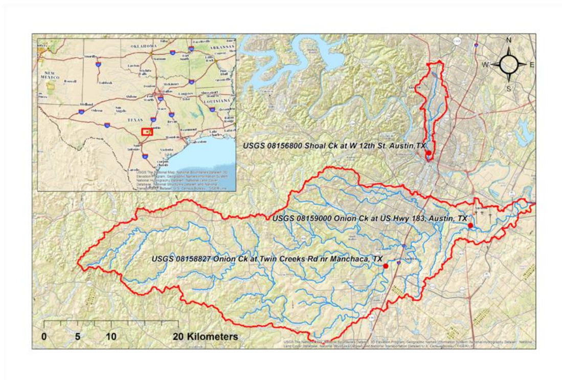
Figure 2.1 Map of Onion Creek and Shoal Creek watersheds as well as USGS gages used to compare with model results.
