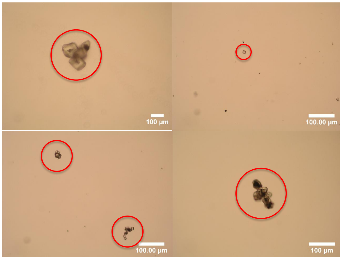
Figure A-20: Crystalline, translucent structures containing opaque particles seen under light microscopy in controls (circled in red). The translucent, crystalline structures are predicted to be calcite, and the opaque particles are predicted to be CuO NPs. Clockwise from top left: alkalinity control, alkalinity control, control, control.
