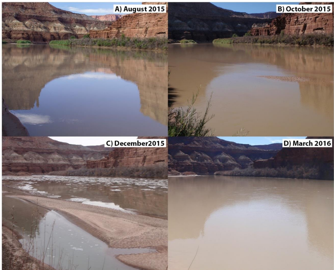
Figure 2.13: A photo match taken at the Hardscrabble trench, showing offshore bar deposition and erosion in summer and fall low flows. Photos are looking downstream. A) Photo taken August 7, 2015 at 2,610 \text{ ft}^3/\text{s} , B) Photo taken October 15, 2015 at 2,640 \text{ ft}^3/\text{s} , C) Photo taken December 6, 2015 at 2,820 \text{ ft}^3/\text{s} and D) Photo taken March 2016 at 3,400 \text{ ft}^3/\text{s} . Discharge values are from the Mineral Bottom gage. The highest flow in this time period was 6,650 \text{ ft}^3/\text{s} on October 20, 2015.
